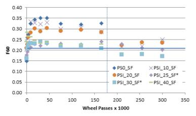
Effect of local coarse aggregate content (0% to 40%) on frictional properties of dense graded asphalt with steel slag coarse aggregate.
