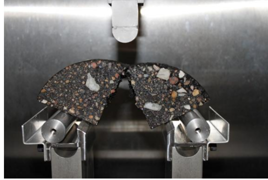
(b) SCB specimen with fracture
