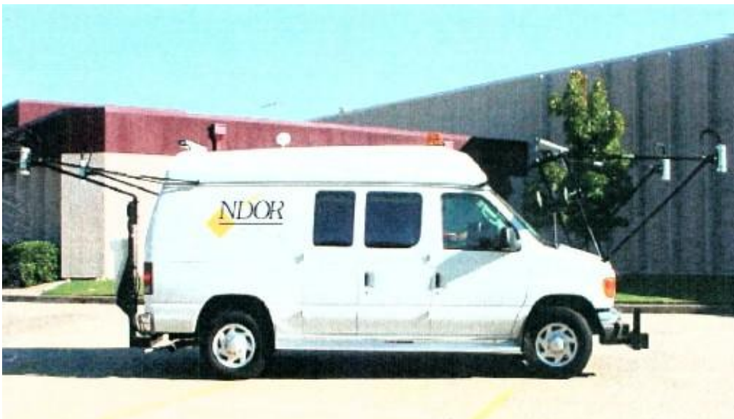
Figure 3.22 A Vehicle Used to Monitor Pavement Performance
