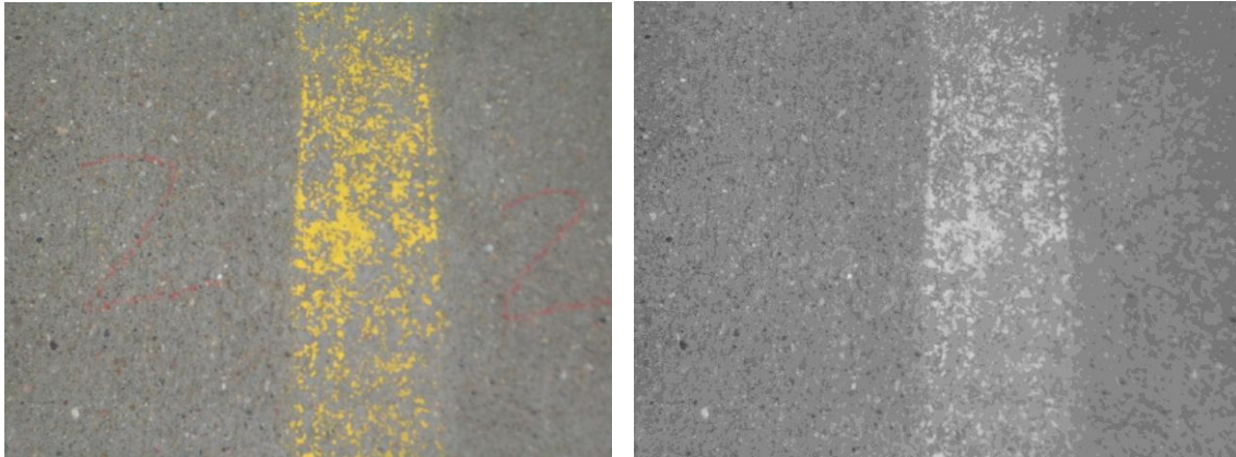
Figure 7.1 Actual picture (on left) and grayscale image (on right) of pavement after marking has been removed
