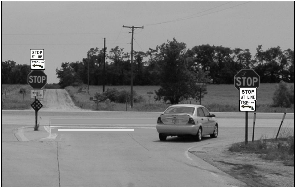
Figure 9.29 Simulation of Proposed Single-Signing Recommendation
