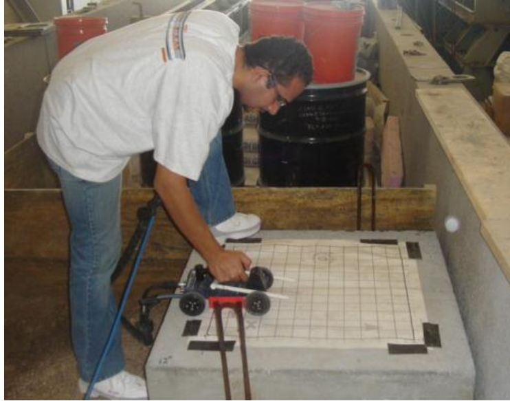
Figure 3.2 GPR grid scan of the 12 in. thick concrete slab
