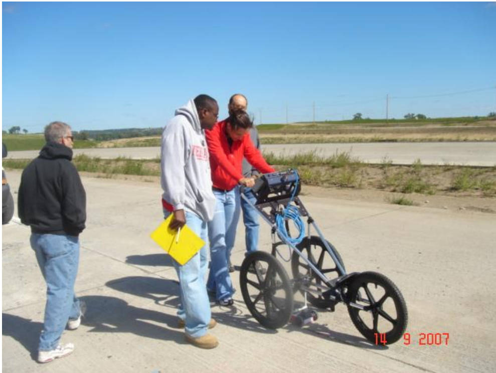
Figure 4.1 GPR scan using the SIR 3000 system on Highway I-275
