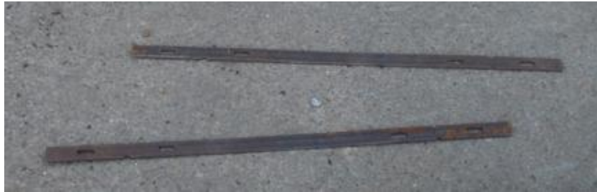
Figure 3.6 Form ties used in the lab test # 1
