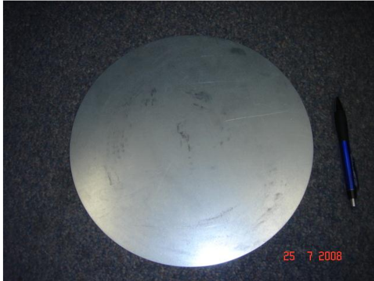
Figure 4.15 Steel plate placed underneath the concrete pavement
