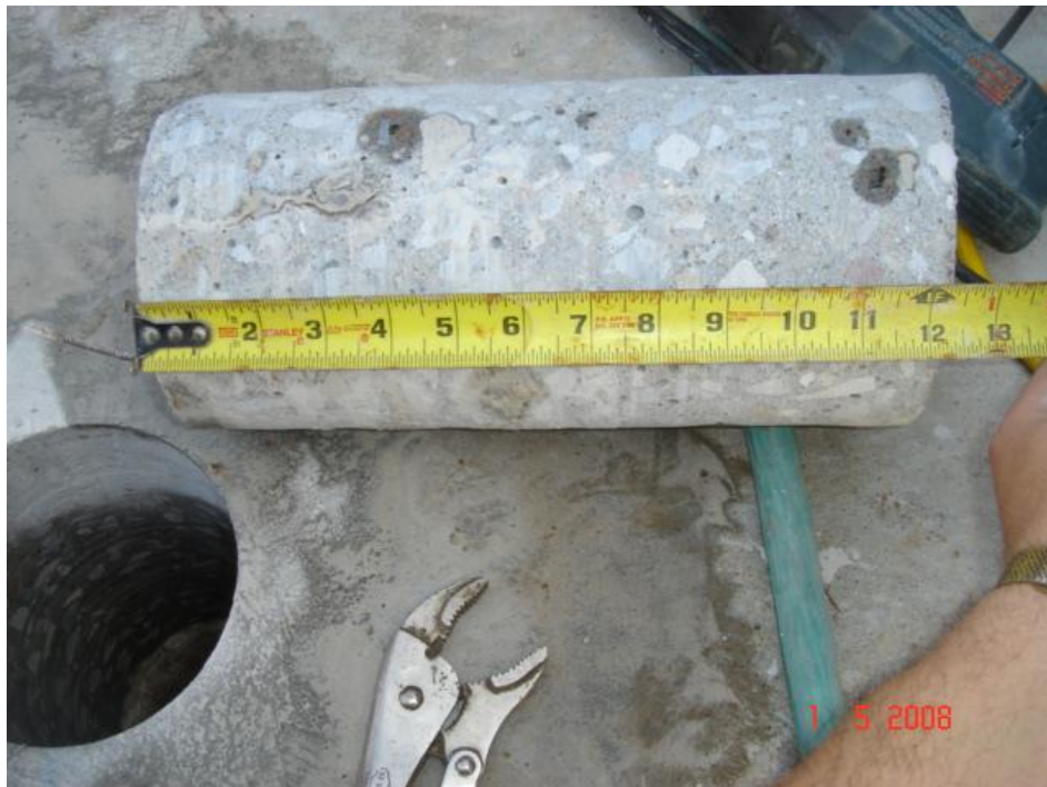
Figure 3.16 Thickness measurement using extracted cores
