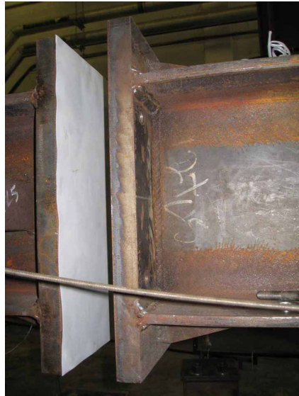
Figure 7-22. Teflon sheet placed between flange plates
