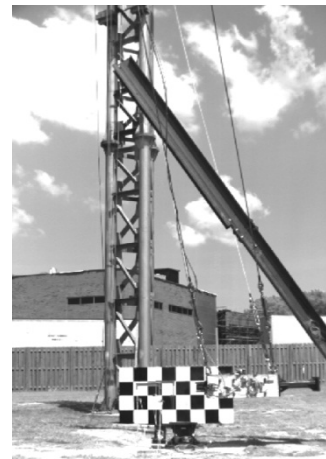
Figure 10-31. Head-on impact from high-speed camera (where t = 0 \text{ sec.} indicates contact between post and pendulum) for experiment T-0-1
