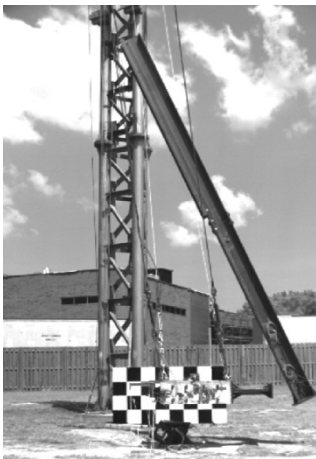
Figure 10-31. Head-on impact from high-speed camera (where t = 0 \text{ sec.} indicates contact between post and pendulum) for experiment T-0-1
