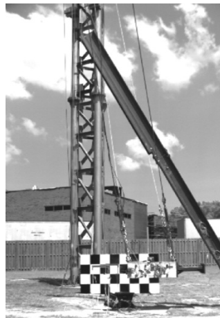
Figure 10-31. Head-on impact from high-speed camera (where t = 0 \text{ sec.} indicates contact between post and pendulum) for experiment T-0-1
