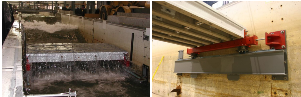
Figure 3: Hydrodynamic 1/5-scale model of bridge span in wave flume (Bradner, 2008).
