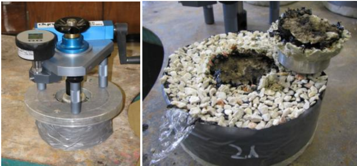
Figure 3. Surface Treatment Bond Test Equipment Set-Up and Tested Lab Specimen.
