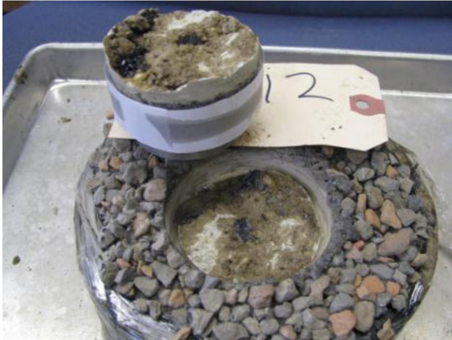
Figure 3.5. Failure Plane of Surface Treatment Bond Test when Prime Coat A Material Was Used (Good Penetration of the Prime, Failure in Base Course).
