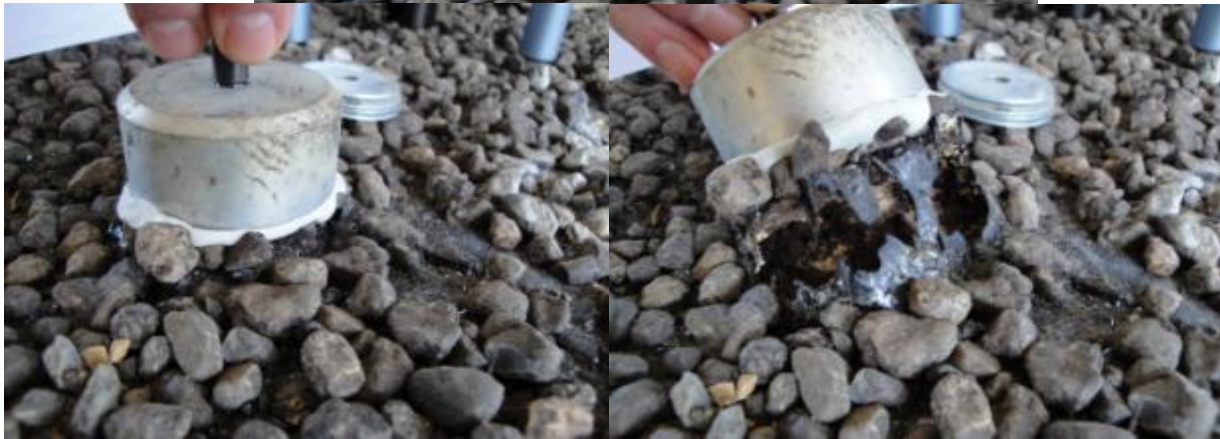
Figure 3.18. Surface Treatment Bond Testing on SH 6.
