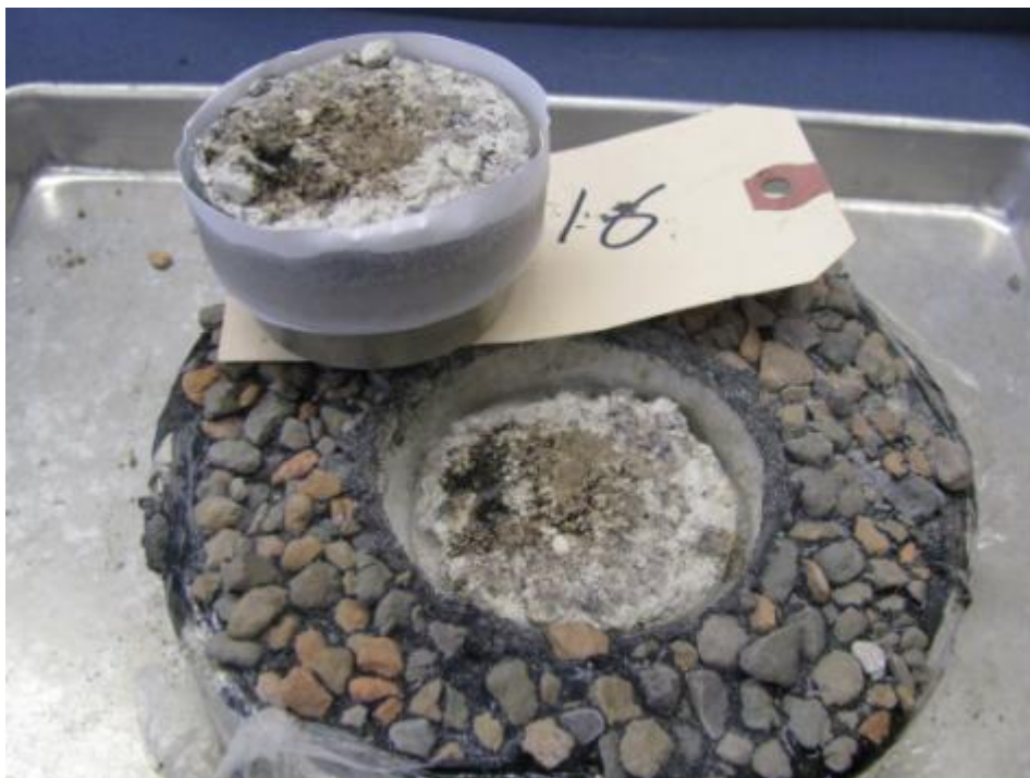
Figure 3.6. Failure Plane of Surface Treatment Bond Test when Prime Coat C Material Was Used (Poor Penetration of the Prime, Failure at Surface Treatment/Base Interface).
