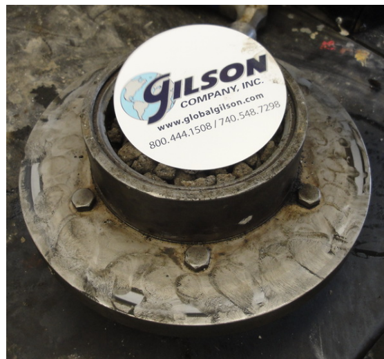
Figure 5. Placement of a Paper Gasket on Top of the Mixture.
