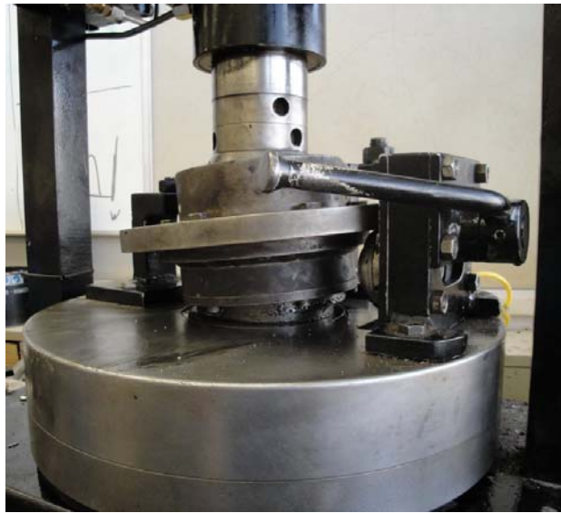
Figure 6. Compaction of Mold Using the TGC.
