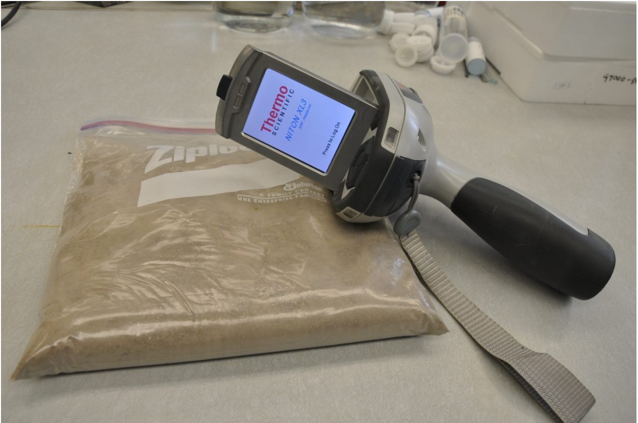
Figure 2.4. Portable Handheld XRF Analyzer and a Soil Sample Used in Study.
