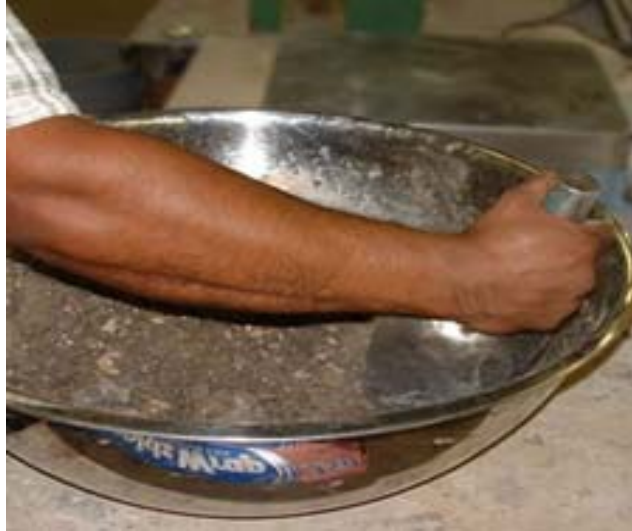
Figure 2. Mixing FDR Materials and a Stabilizer.
