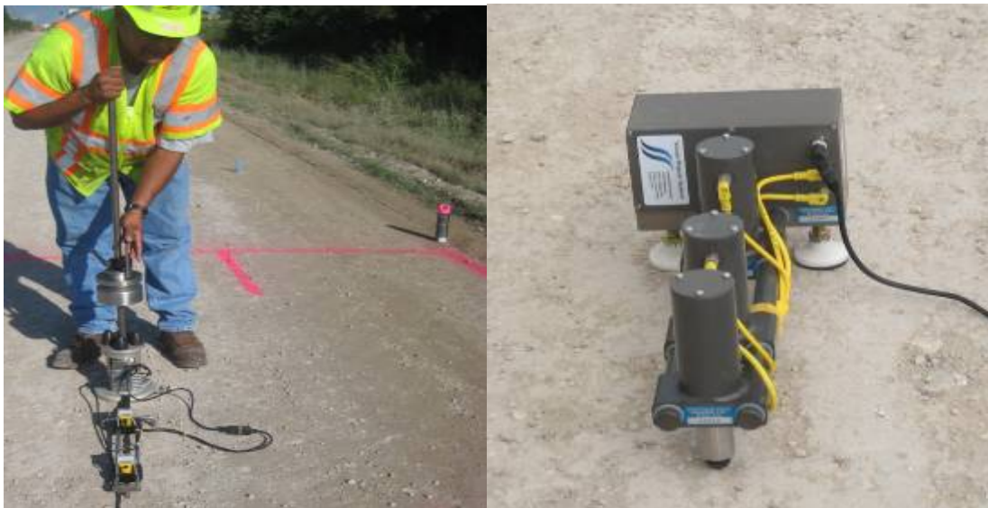
Figure 2.19. Portable FWD and Seismic Test Equipment.
