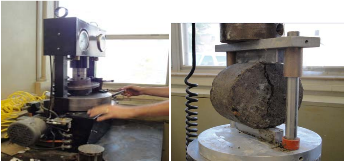
Figure 1.2. Use of the Texas Gyrotory Compactor and IDT Test for FDR Design.
