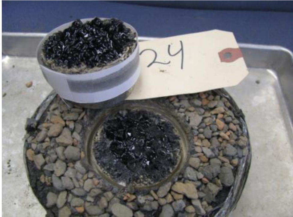
Figure 3.7. Failure Plane of Surface Treatment Bond Test when Covered Prime Was Used (Failure within Surface Treatment Binder Indicating Good Bond to Base Course).
