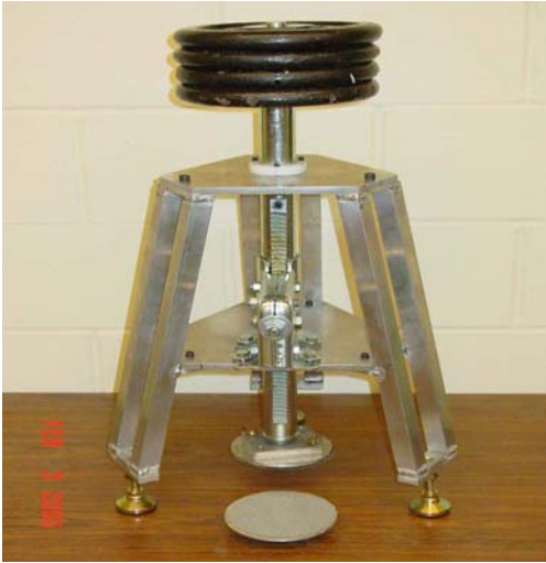
Figure 3.2. Tack Coat Adhesion Tester (Tex-243-F).
