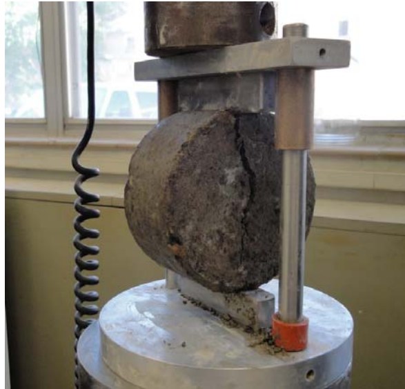
Figure 8. Indirect Tensile Strength Test.
