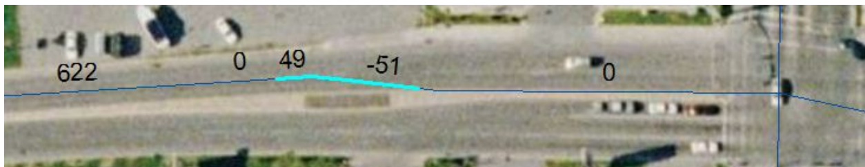
Figure 4-4. Example of radius data caused by van maneuver (radius in feet shown in black).
