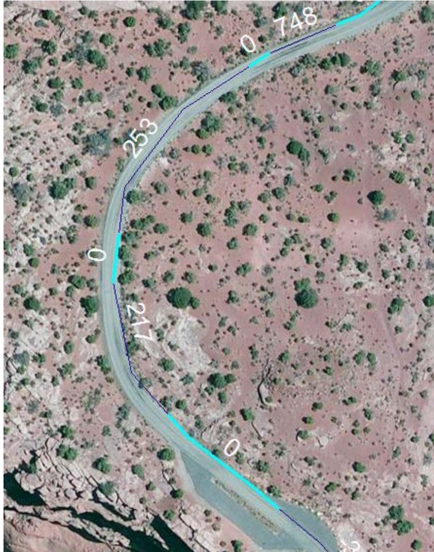
Figure 4-2. Example of inconsistencies in existing geometry data (radius in feet is shown in white).
