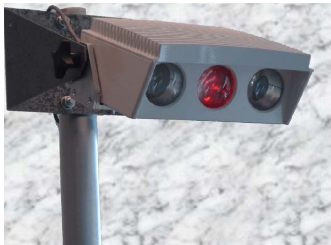
Figure 2.12: Sensice Ice Detector
