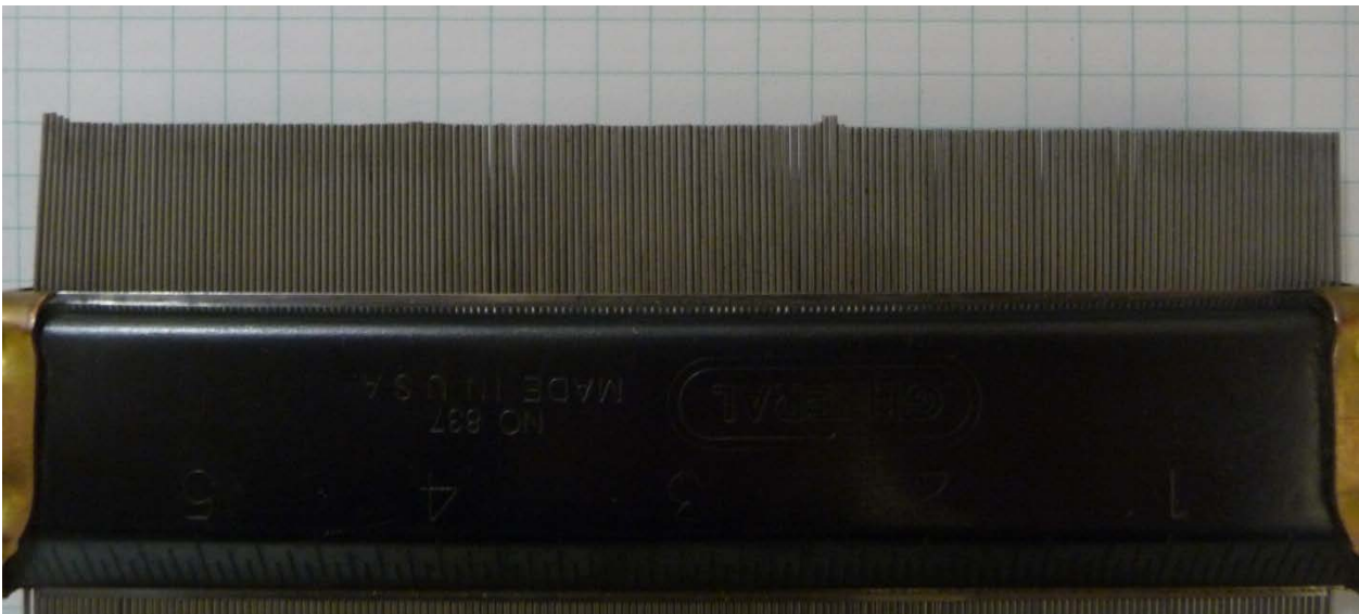
Figure 5.8: Typical asphalt sample surface profile
