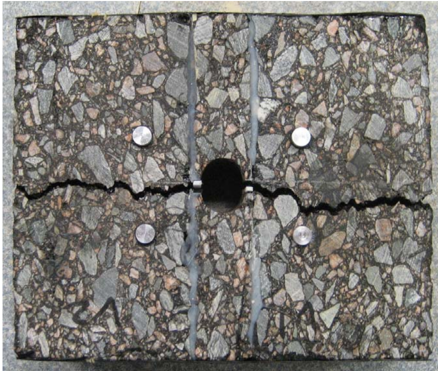
Figure 3-2. Typical failure mode of composite specimen
