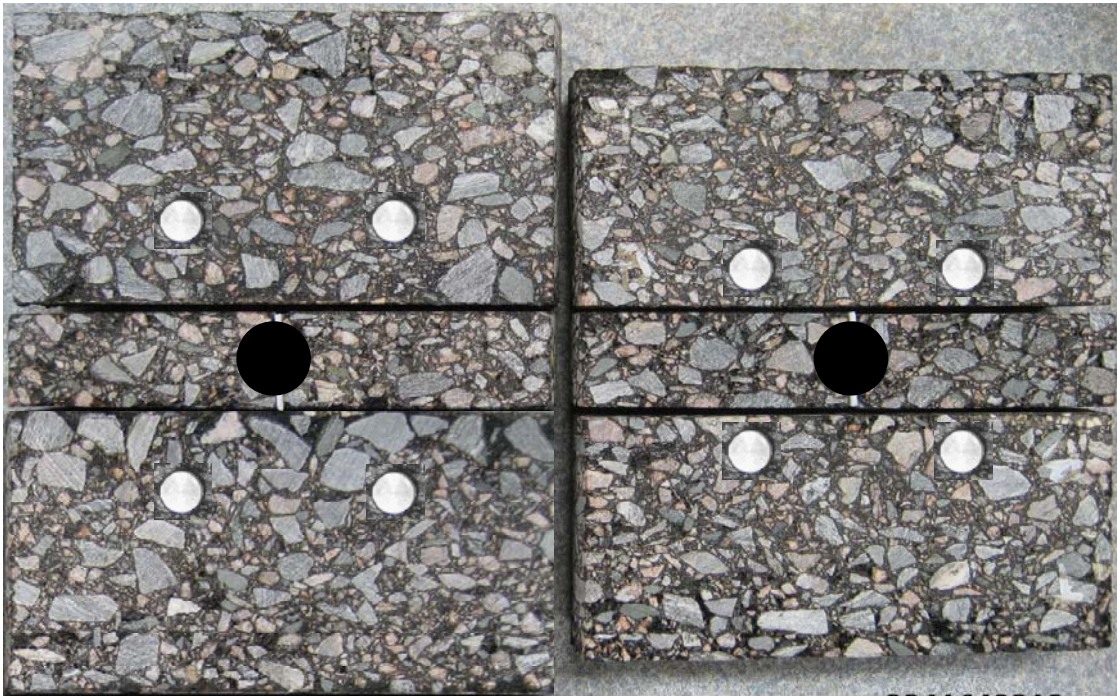
Figure 2-2. Typical composite specimens with ARMI layer (left) and without ARMI layer (right) ready to be glued together with epoxy
