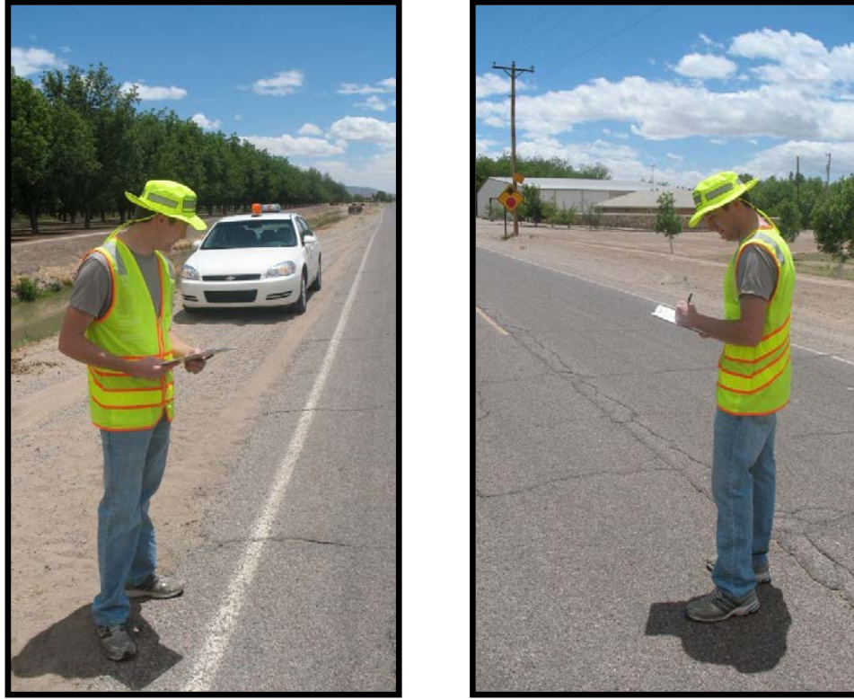
FIGURE 7 An NMSU rater performs visual distress survey of a flexible pavement section, walking from (left) and to (right) the vehicle
