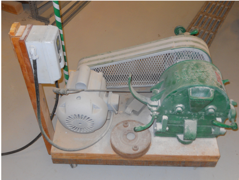
Figure 2-2: Pulverizer at Oregon State University
