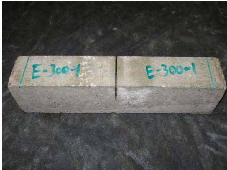
(b) Notched sample cut by diamond saw
