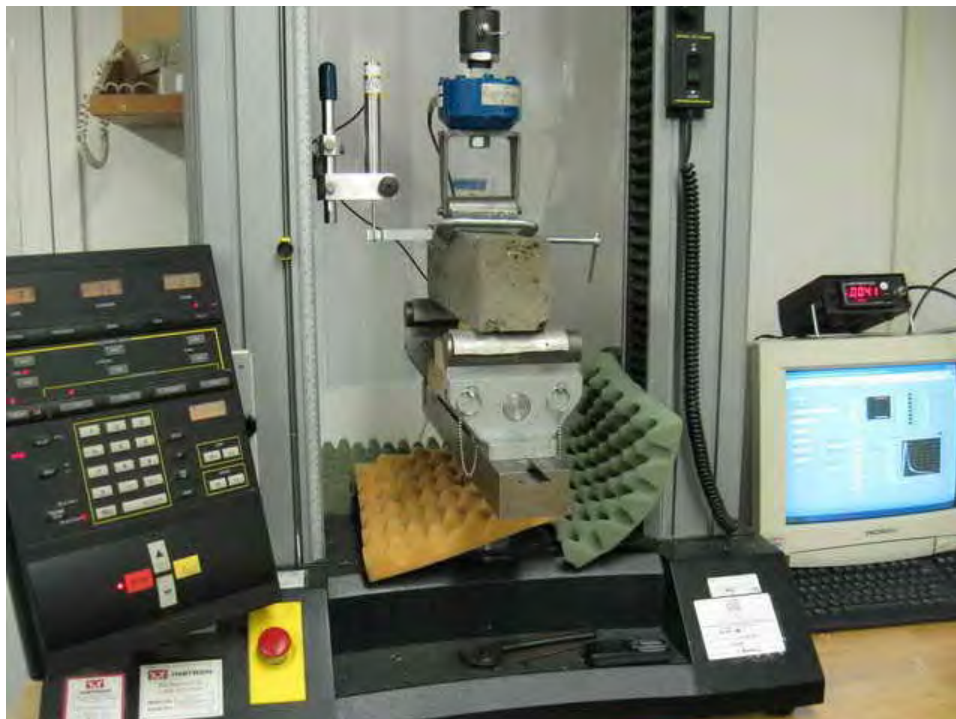
Figure 3.12 Testing Equipment Setup for Fracture Test.
