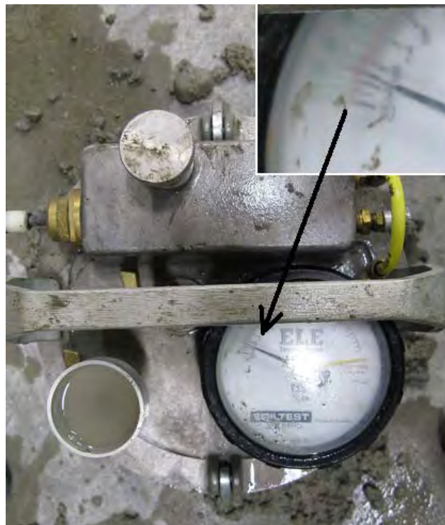
Figure 3.2 Air Content Test
