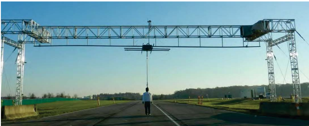
Figure ES 2: Test Apparatus Used to Simulate Pedestrian Crashes During Testing
