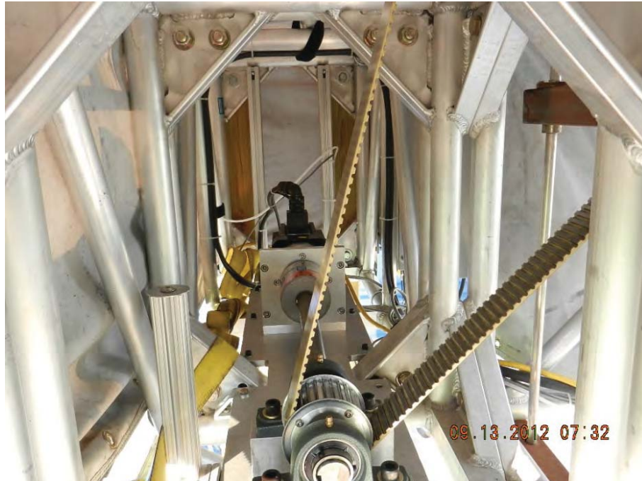
Figure 21: Servo Drive, Gearbox, and Drive Pulley With Improved Mounting System
