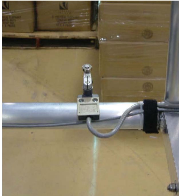
Figure 187: Illustration of End-of-Travel Switch
