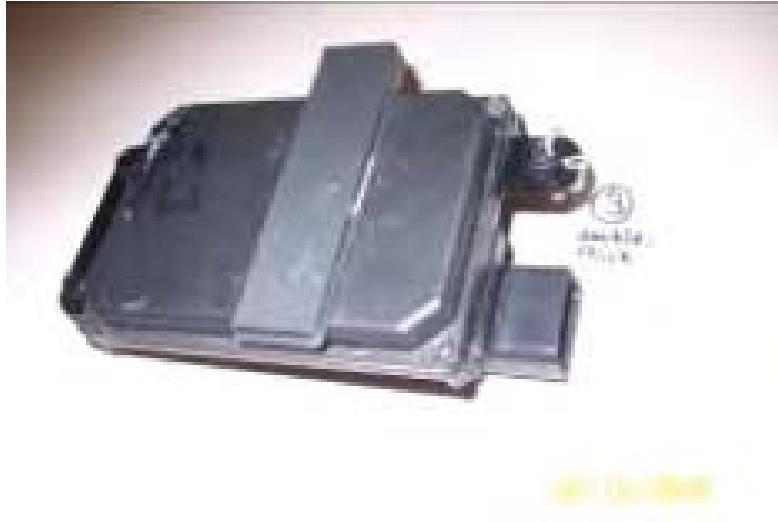
Figure 113: Plastic Strips Used to Emulate Partial Ice Blockage
