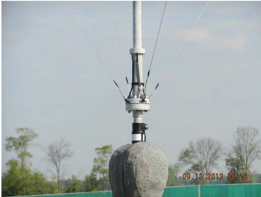
Figure 25: Illustration of Quick-Release Mechanism for Mannequin Attachment to Support Pole
