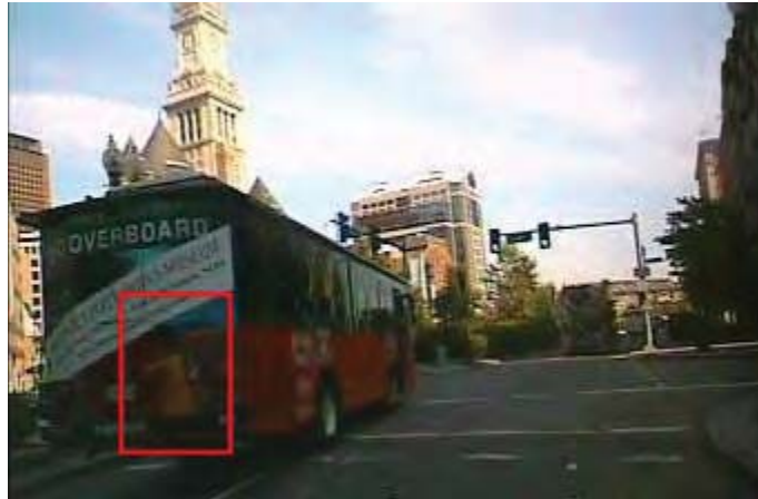
Figure 69: Print of a Person on a Bus Outside of the Vehicle's Travel Lane
