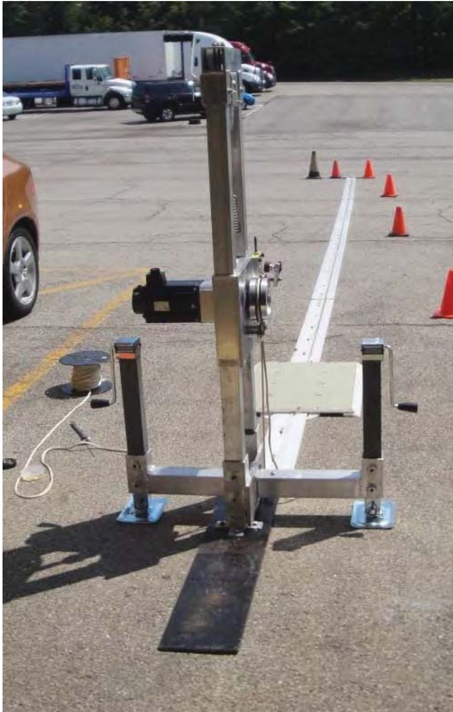
Figure 30: VRTC Ground-Based Apparatus in Crossing Configuration
