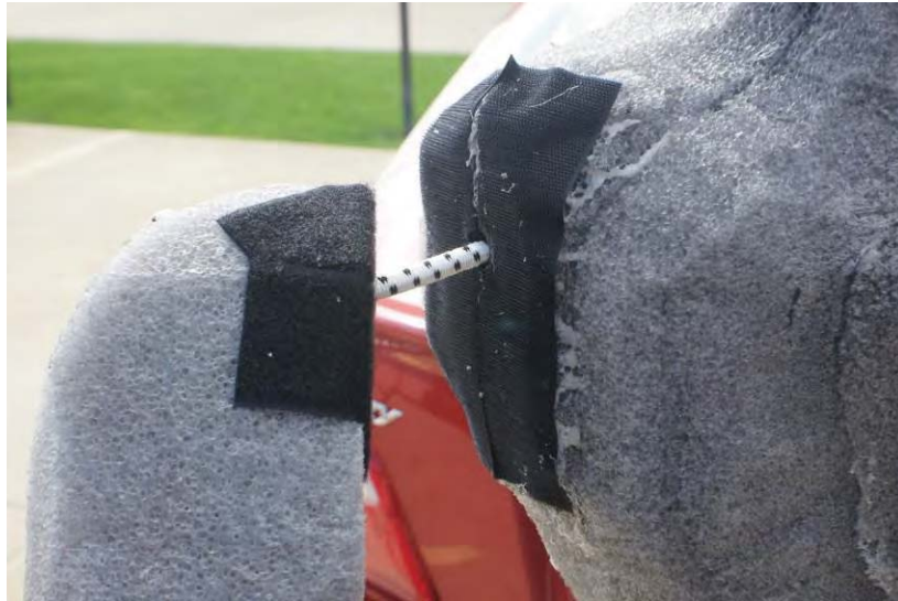
Figure 4: PCAM Mannequin Shoulder Joint Construction
