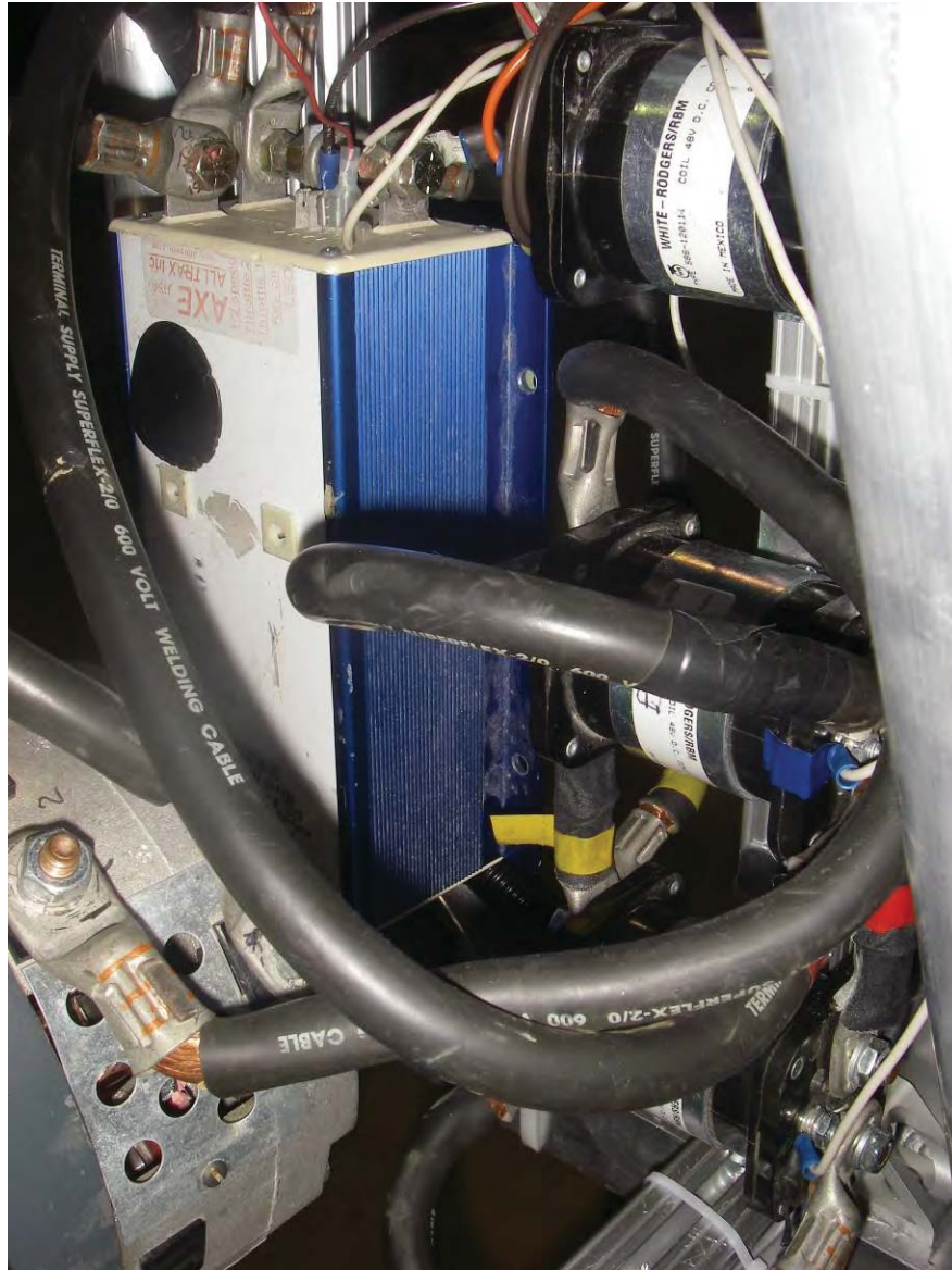
Figure 185: Illustration of the Controller With Contactors
