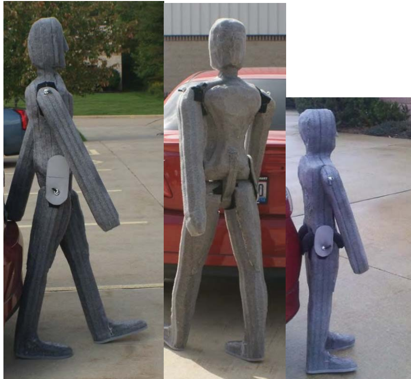
Figure 5: Illustrations of Pedestrian Mannequins: Adult Mannequin (Left and Center Photos) and Child Mannequin (Right Photo)
