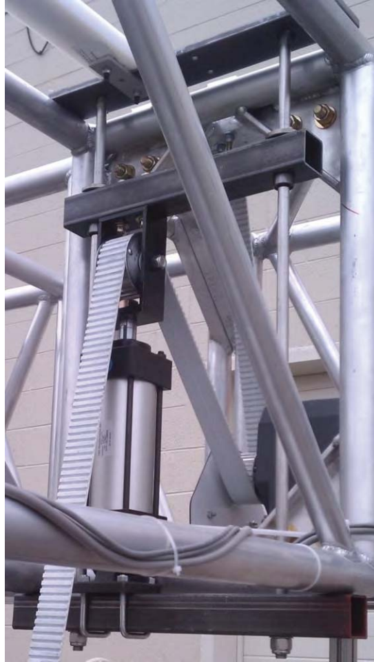
Figure 182: Illustration of Drive Pulley (lower right) and Tensioner Assembly (left)
