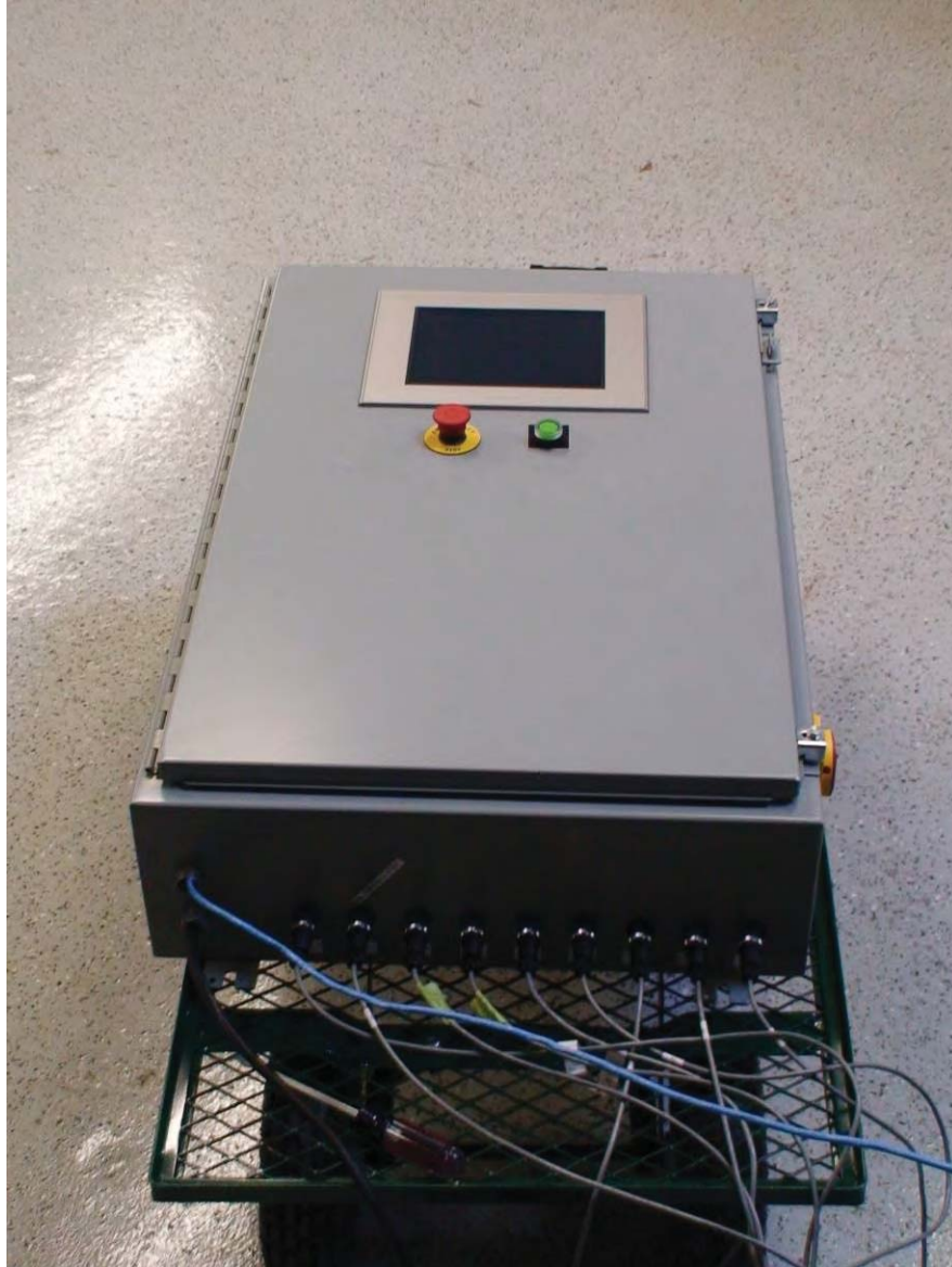
Figure 188: Illustration of Control Box With Emergency Stop Button and Touch Screen
