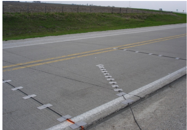
Figure B-3. Road tube layout to measure lane positioning in the field
