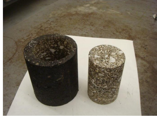
Figure 4.1. A Specimen Cored and Sawn from the Gyratory Compacted Sample
