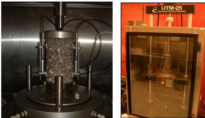
Figure 4.3. A Specimen with LVDTs Mounted in the UTM-25kN
