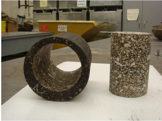
Figure 4.1. A Specimen Cored and Sawn from the Gyratory Compacted Sample
