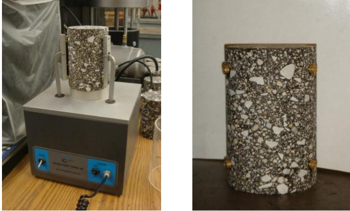
Figure 4.2. A Device Used to Place the Mounting Studs for LVDTs
