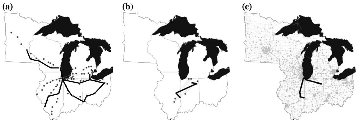
Figure 2.4 (a) rail network in study region (Amtrak in gray, HSR in black); (b) maximum utility rail paths (showing connectivity, not geographic path) for stations near Edgar County, IL and Kosciusko County, IN; (c) maximum total utility path between origin and destination county
