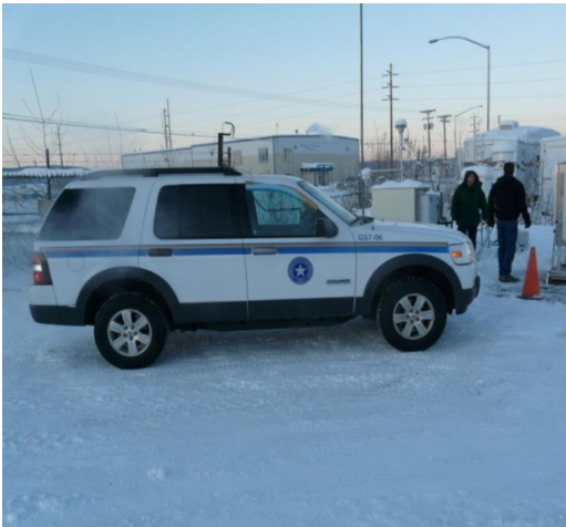
Fig. 1. Mobile platform and its outside measurement equipment. The 2007 FNSB-owned Ford Explorer is equipped among other things with a data RAM4000 monitor, BGi \text{PM}_{2.5} sharp cut cyclone, sample liner heaters, Garmin GPS, DryCal flow calibrator, temperature loggers, and a 300W power converter. Courtesy to F. di Genova [2009]
