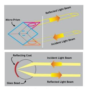
Retroreflection is achieved through either glass beads or microprisms imbedded in the sheeting.
