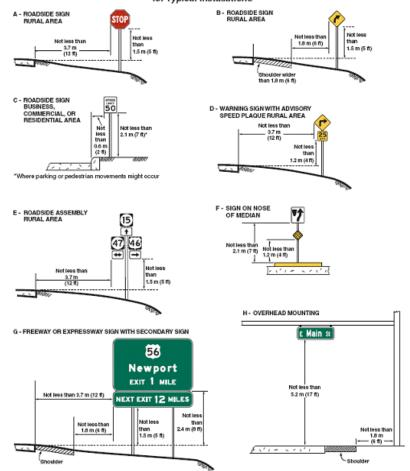
Figure 2A-2. Heights and Lateral Locations of Signs for Typical Installations
