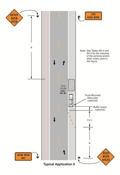
3. Typical Traffic Control Layout for Mobile Operations on Two-Lane Road
