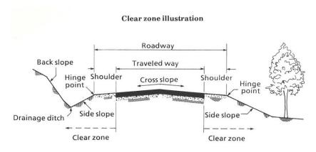
Point where the slope rate changes. Hinge Point
