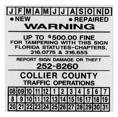
Sign dating labels with anti-vandalism warnings can be applied to the back of the sign.
