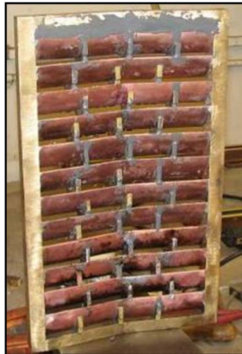
Figure 3.6 Type 16 Grate During Fabrication
