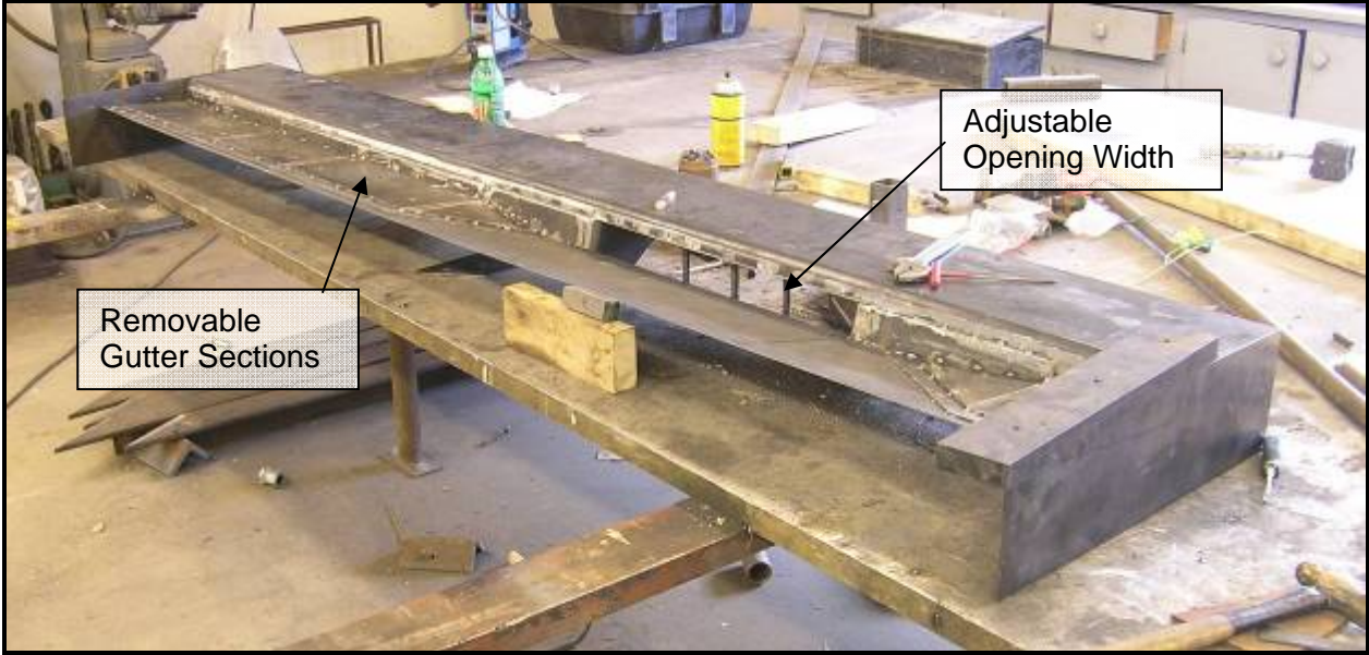
Figure 3.3 Curb Inlet Gutter Panel During Fabrication (Type R)
