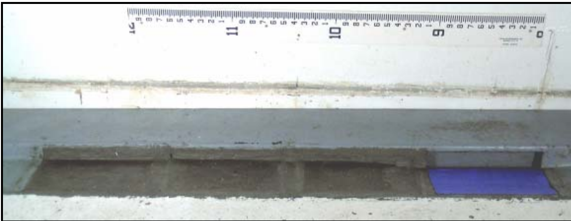
Figure 3.12 Single No. 13 Curb Opening Only Photograph
