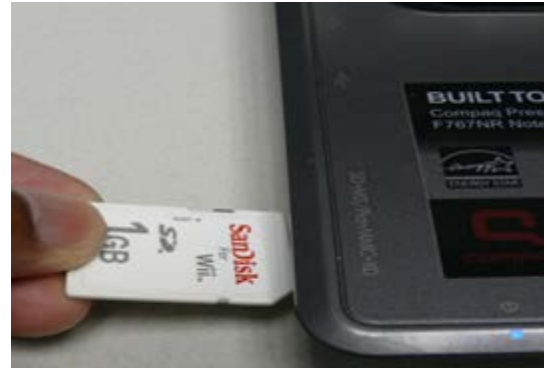
Figure A-1. Insert SD Card into SD Drive on the Computer.
