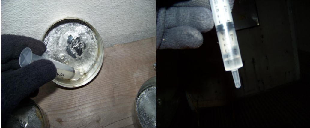
Figure 3.16 Refreeze Test liquid measurement
