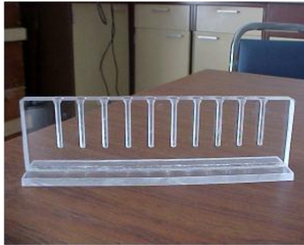
Figure 2.2 Ice penetration test apparatus (Nixon et al. 2007)
