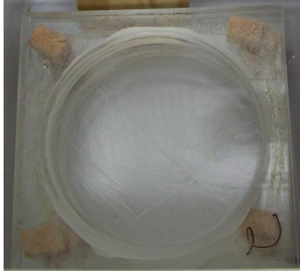
Figure 2.1 Ice melting capacity dish
