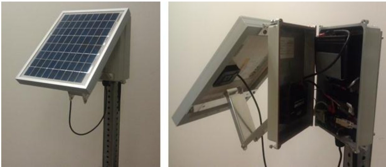
Figure 10. Roadside data collection unit
