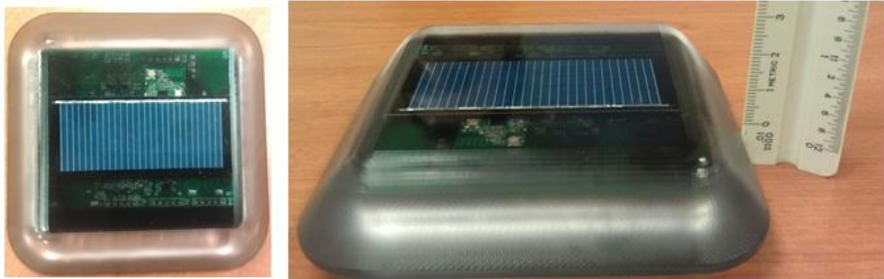
Figure 7. Wireless traffic sensor in Lexan enclosure
