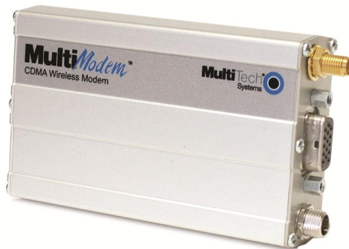
Figure 9. Wireless modem for real-time data transmission
