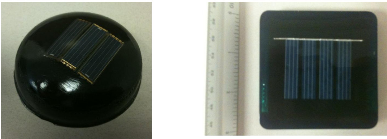
Figure 3. Protecting the electronic parts using a weather resistant epoxy
