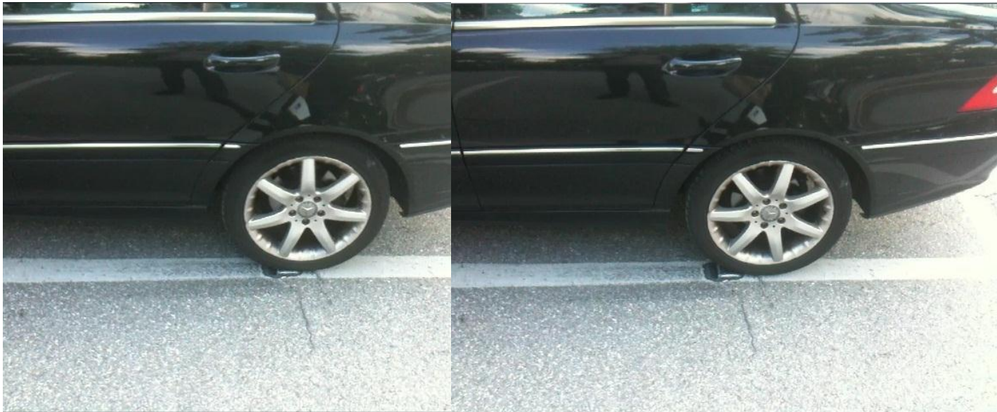
Figure 8. Enclosure resistance test under real road conditions
