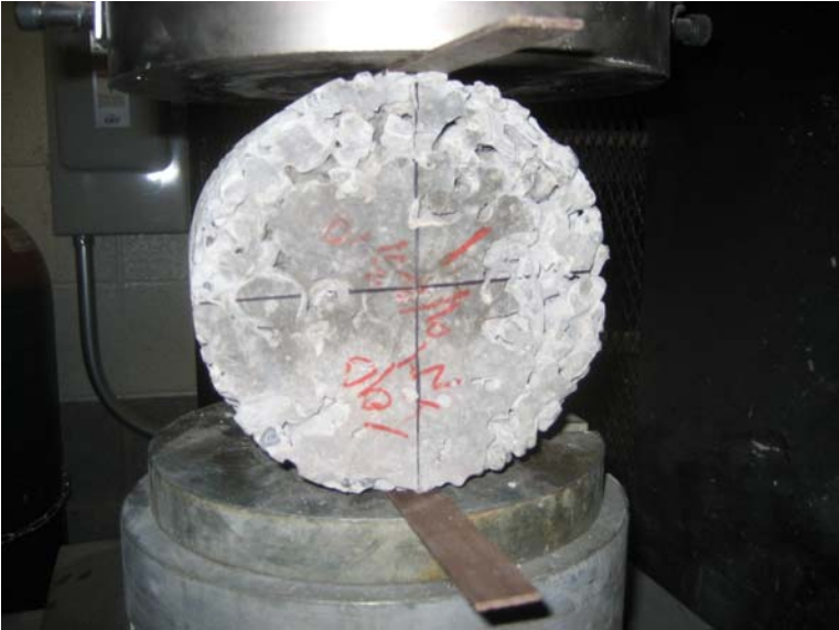
Figure 18 Split-cylinder tensile test setup on CTPB sample
