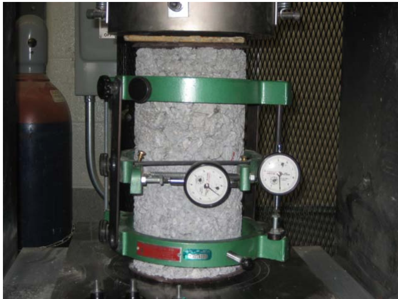
Figure 17 Static modulus and Poisson's ratio test setup for CTPB specimen
