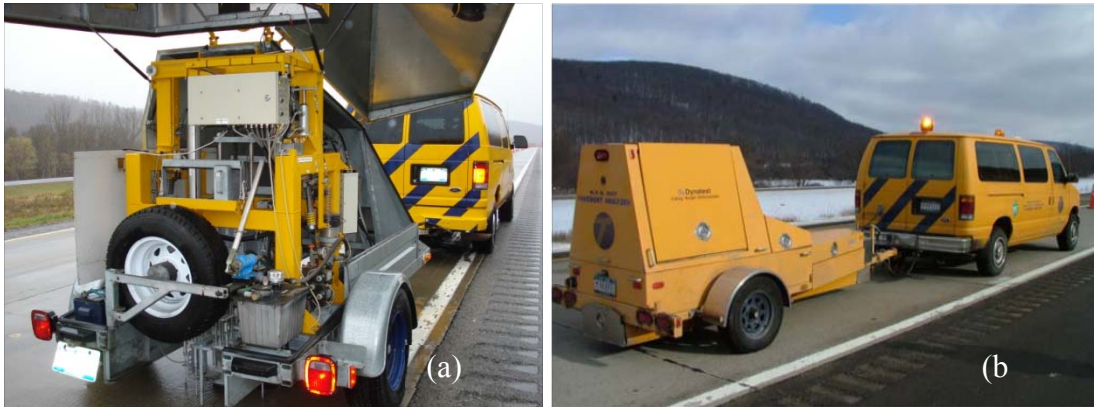
Figure 9. Falling Weight Deflectometer Systems used by NYSDOT: a) KUAB 120 SP1G; b) Dynatest Model 8000.
