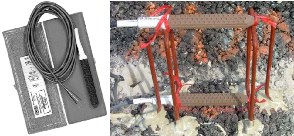
Figure 7. Vishay EGP-5-120 Strain gauge. Left: Standard gauge [Vishay, 2006]; Right: As installed [Ambrosino, 2007].
