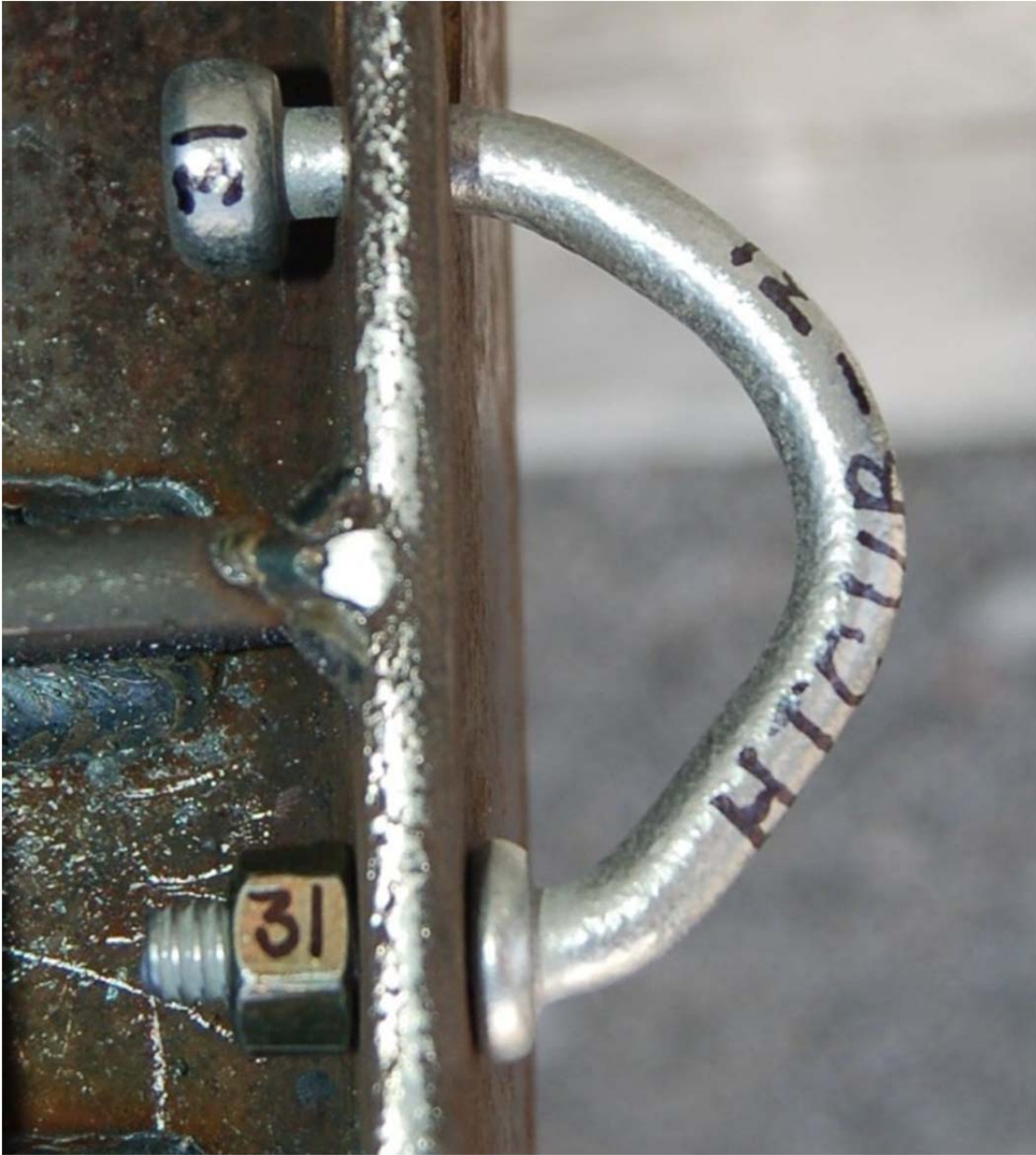
Figure 2. Updated Cable Attachment: Angled Keyway Bolt
