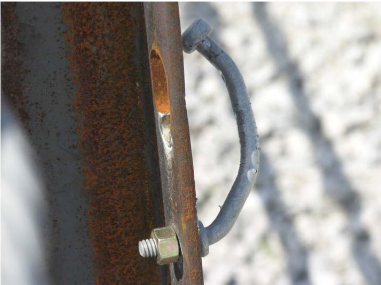
Figure 82. Post and Splice Damage, Test No. 4CMB-5
