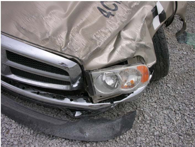
Figure 84. Vehicle Damage, Test No. 4CMB-5
