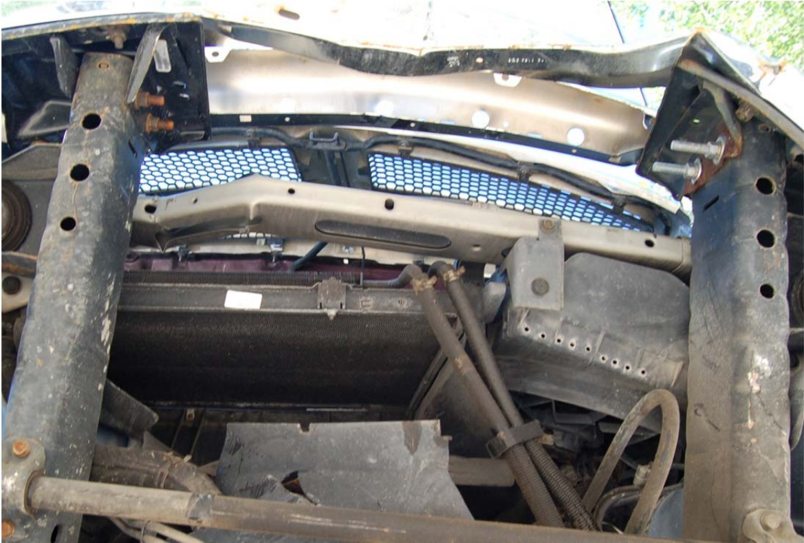
Figure 86. Undercarriage Damage, Test No. 4CMB-5
