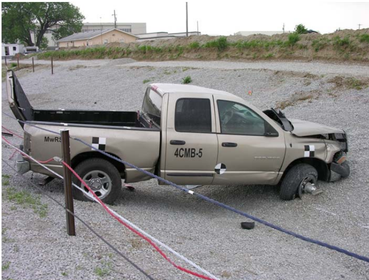
Figure 83. Vehicle Damage, Test No. 4CMB-5
