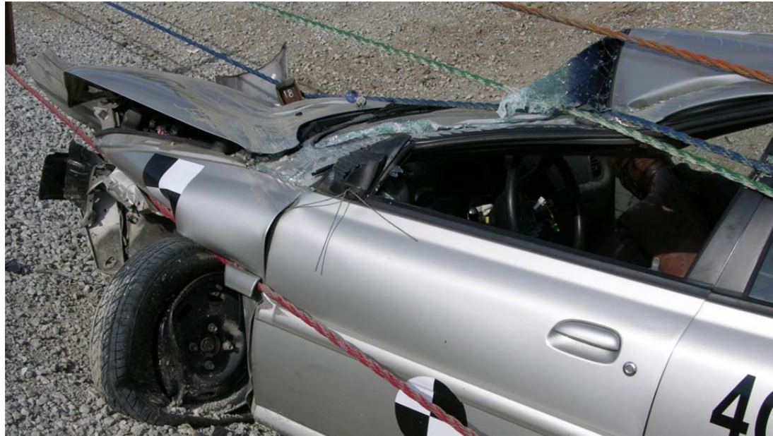
Figure 1. Test No. 4CMB-3: Slotted Bracket, Cable Snag, and A-Pillar Damage
