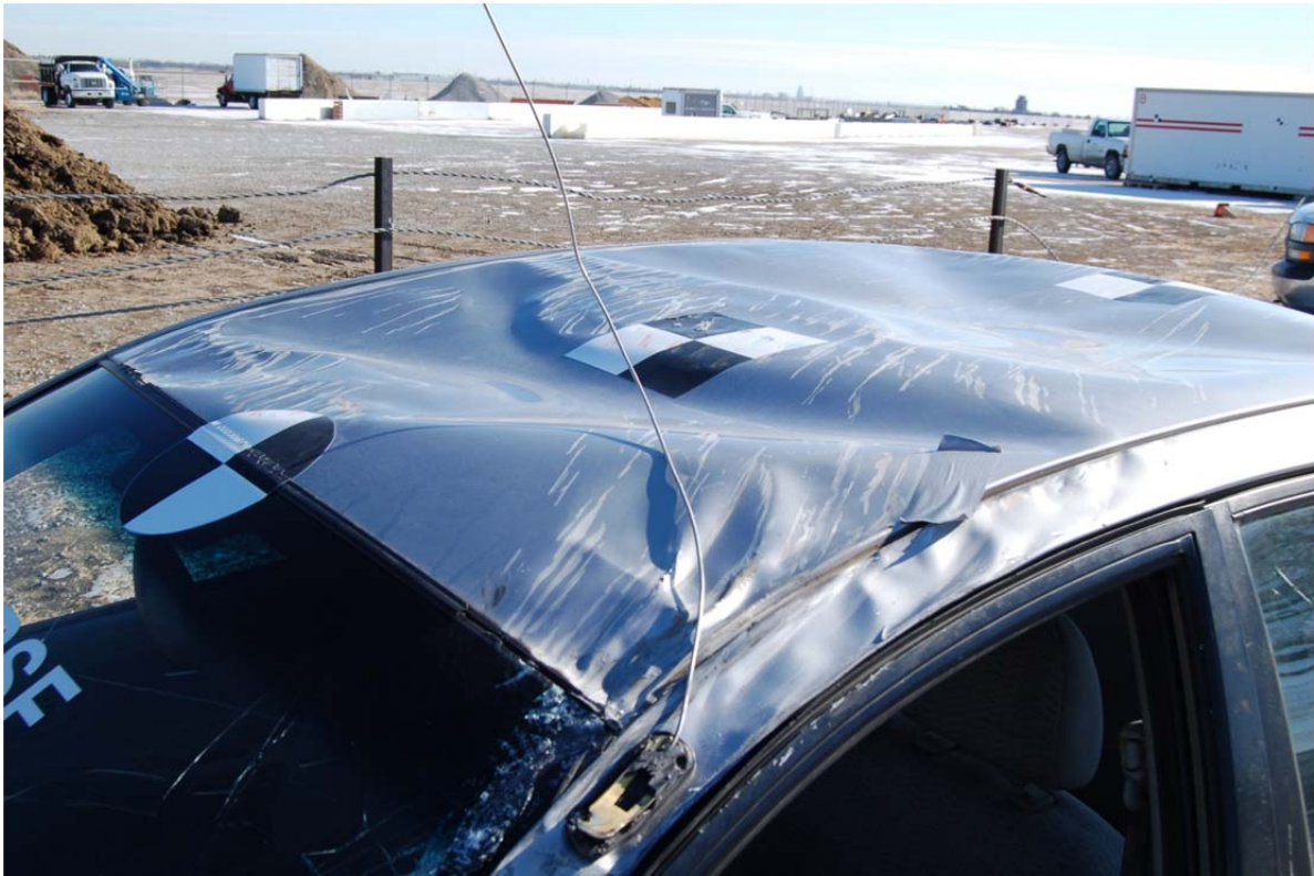
Figure 48. Occupant Compartment Damage, Test No. 4CMB-4
