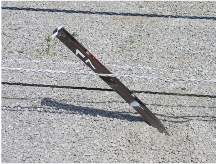
Figure 81. Post Damage, Test No. 4CMB-5
