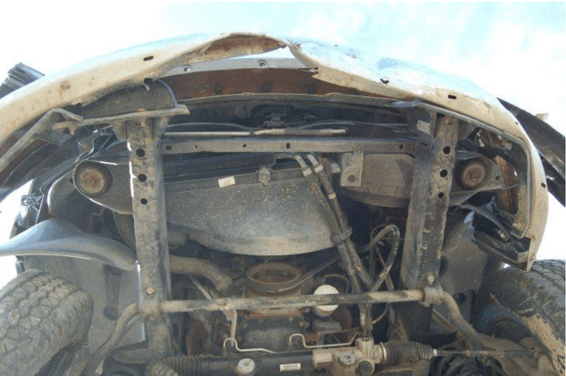
Figure 48. Vehicle Undercarriage Damage, Test No. 4CMB-1
