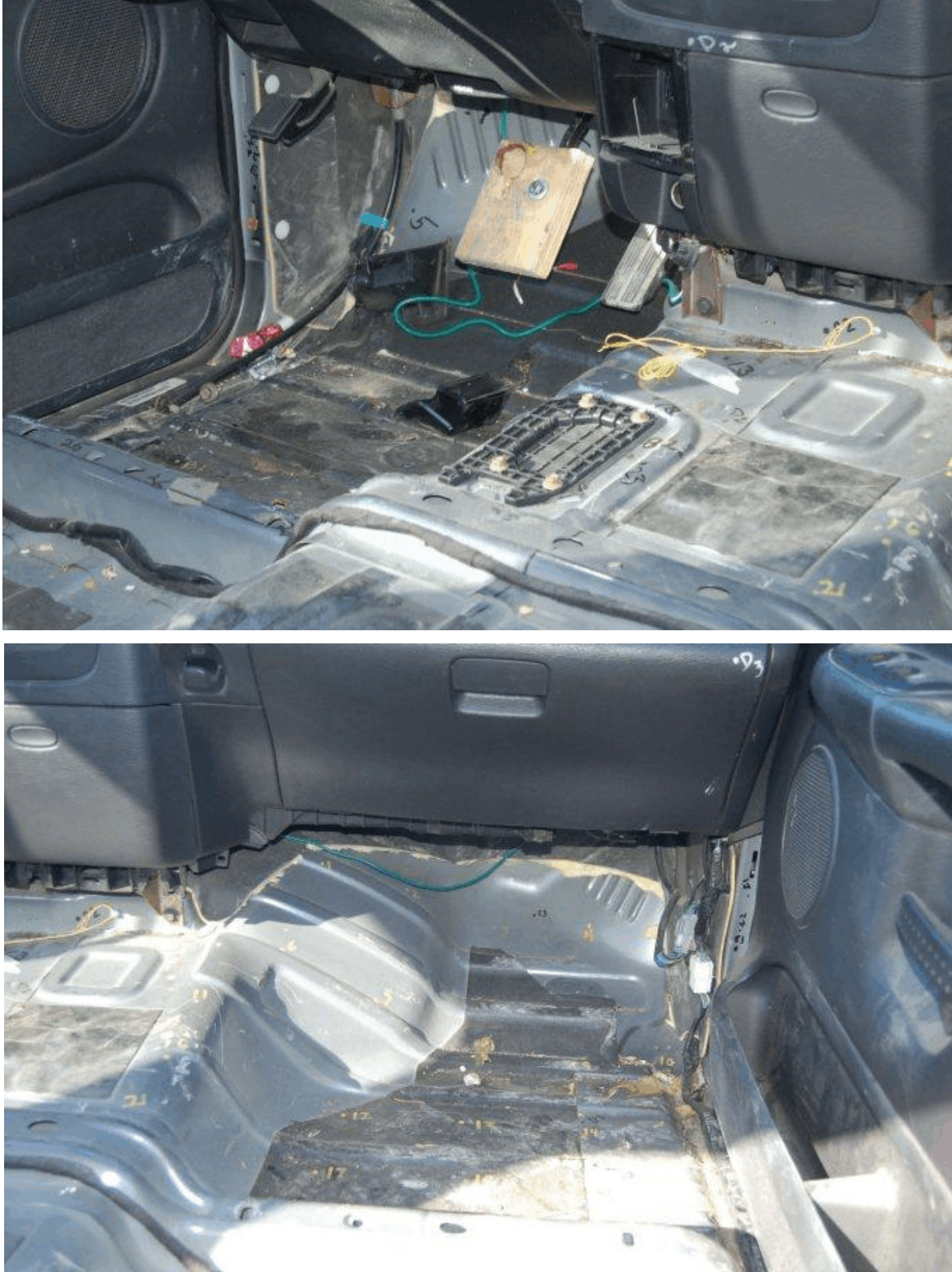
Figure 47. Occupant Compartment Damage, Test No. 4CMB-1
