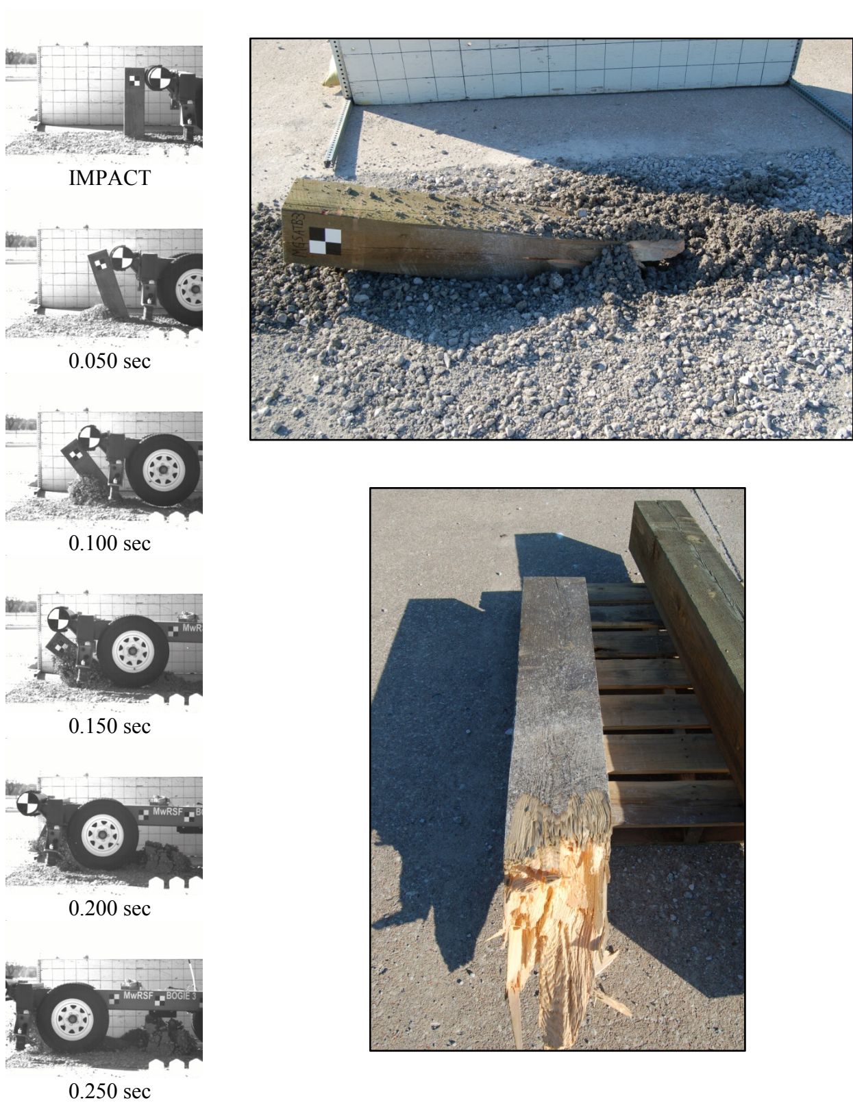
Figure 10. Time Sequential and Post-Impact Photographs, Test No. MGSATB-3
