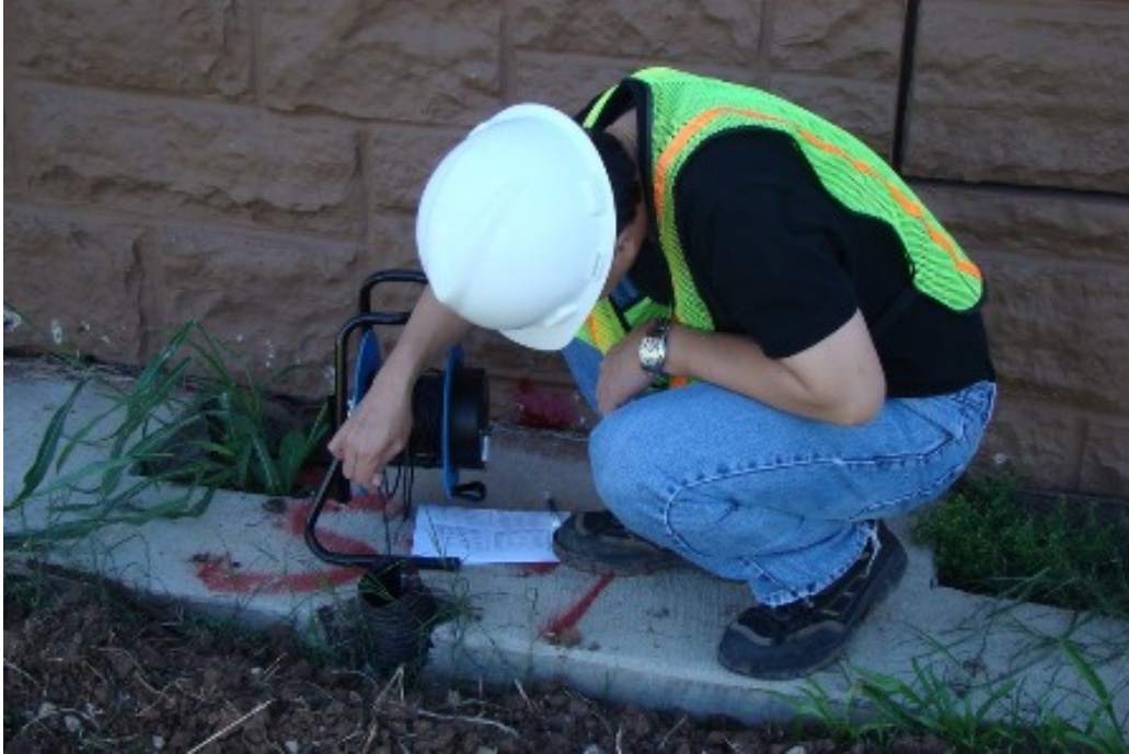
Figure 7.14. The Sondex Instrument and the Readings.
