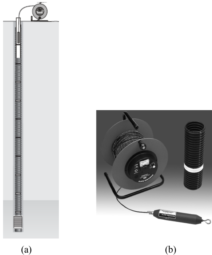
Figure 6.22. (a) A Typical Sondex Installation (b) Sondex System Components (Slope Indicator, 2004).
