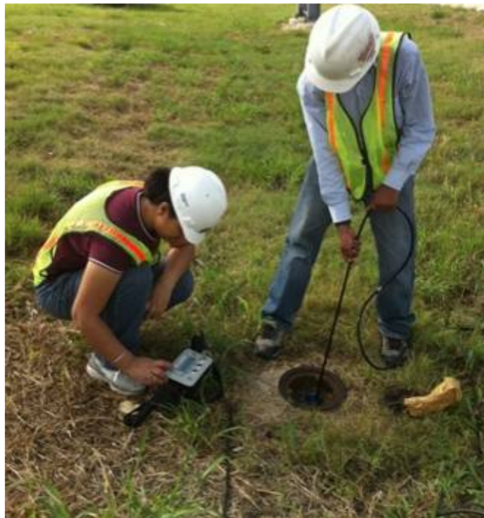
Figure 7.16. The Vertical Inclinometer Reading.
