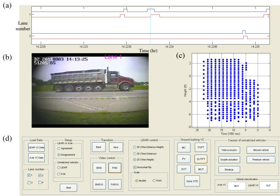
Figure 4-5, A snapshot of the semi-automated GUI verification tool processing a conflicting classification for a vehicle in lane 1 at SR 33 northbound. The GUI window consists of four interfaces: (a) plot of transition pulses, the plot shows for each lane the classification station data (top curve) and LIDAR data (bottom curve) and the current instant is shown with a vertical dashed line, (b) the current video frame, (c) the LIDAR returns from the vehicle in question, and (d) a panel for controlling the review and entering ground truth data. So in this case the GUI is at the second visible pulse in lane 1 (counted from the left hand side) and is ready for the user to assess the data using the buttons on the right of part (d).
