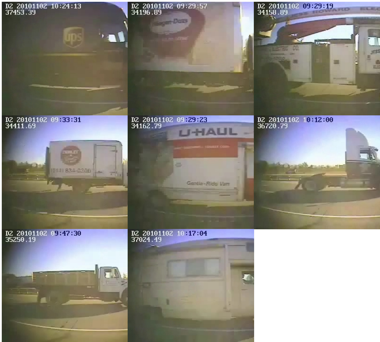
Figure 2-4, Examples of the seven types of two-axle SUT that were misclassified as PV by the axle classification station because the axle spacing fell below the PV boundary.
