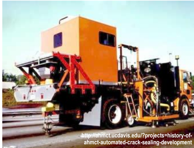
Figure D.15. AHMCT SHRP H107A automatic crack sealing machine, fully operational in 1993
