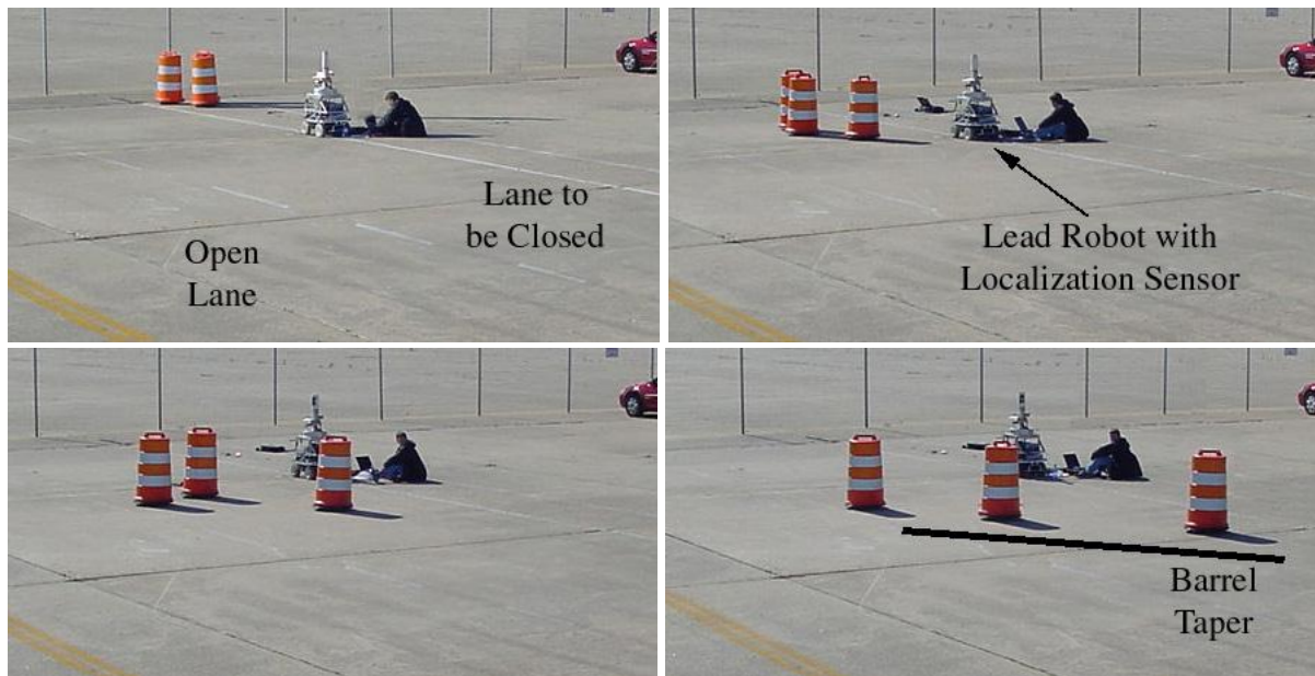
Figure D.18. Lane closure with five barrel robots
