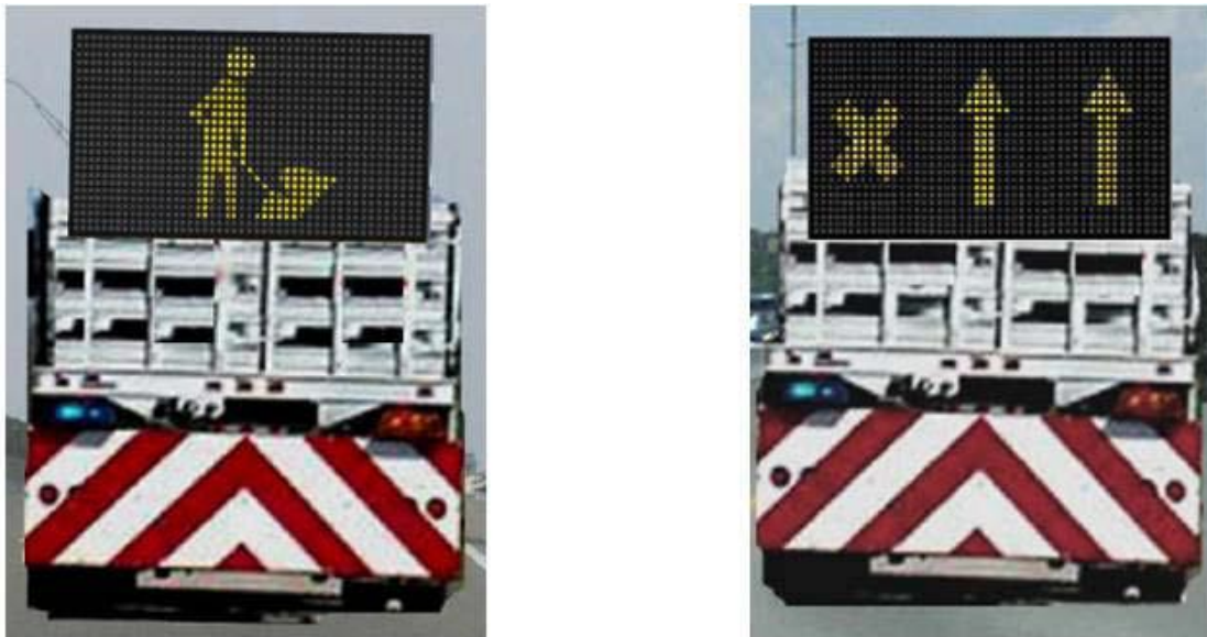
Figure 7. Truck-mounted changeable message signs (event example, left, and lane-blocked example, right) (photos Texas A&M University-Kingsville)
