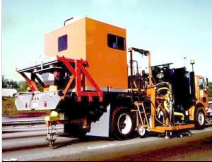
Figure 5. Automated pavement crack sealer
