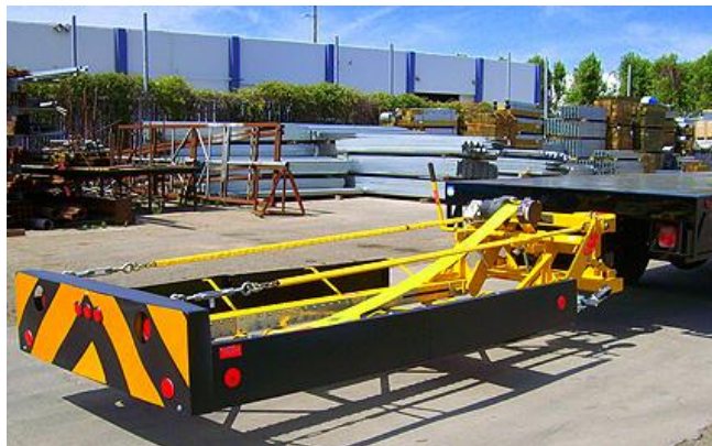
Figure C.4. Truck-mounted traffic attenuator
