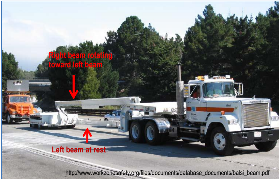
Figure D.2. Second stage: rotating one of the beams to the other side
