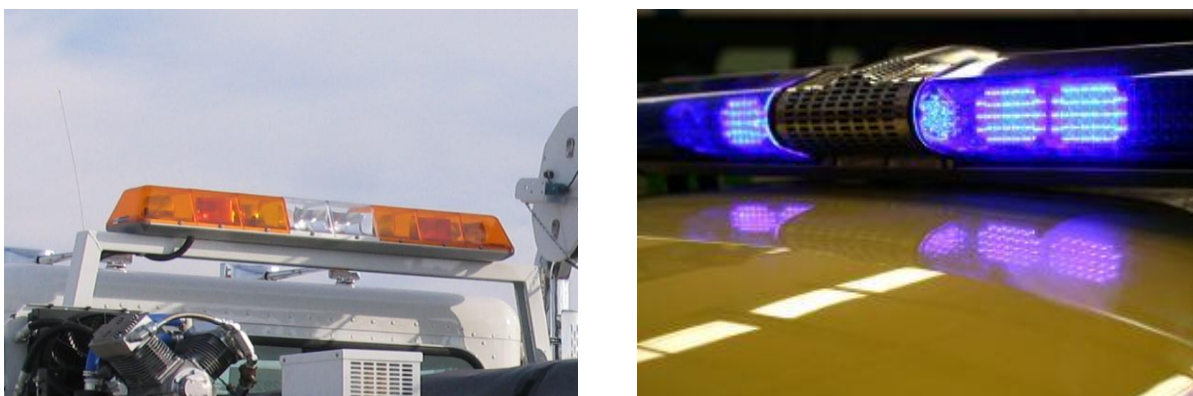
Figure D.9. Amber strobe lights (normally used on work vehicles) (left) and blue strobe lights (recommended for use on work vehicles) (right)
