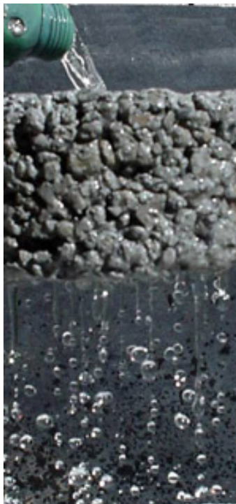
Figure 3.3. Water permeating pervious concrete
