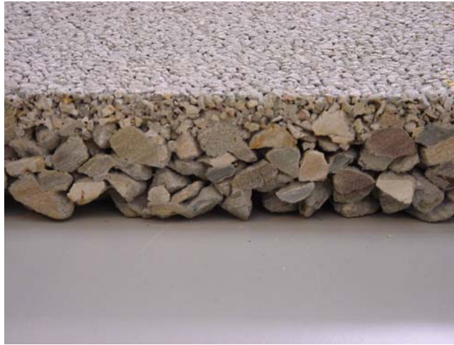
Figure 3.4. Double-layer pervious concrete
