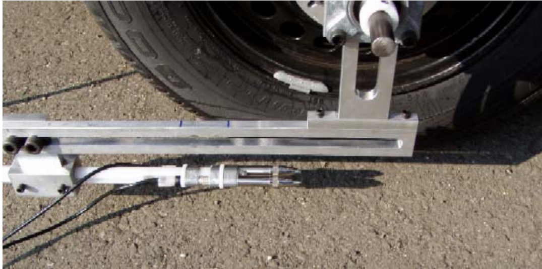
Figure 4.4. OBSI measuring device
