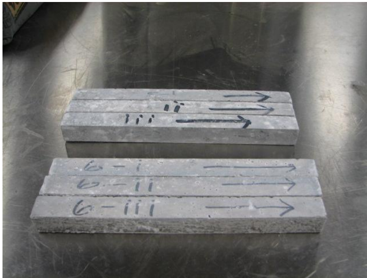
Figure 5.2.8 Mortar Bars following 28 day Testing
