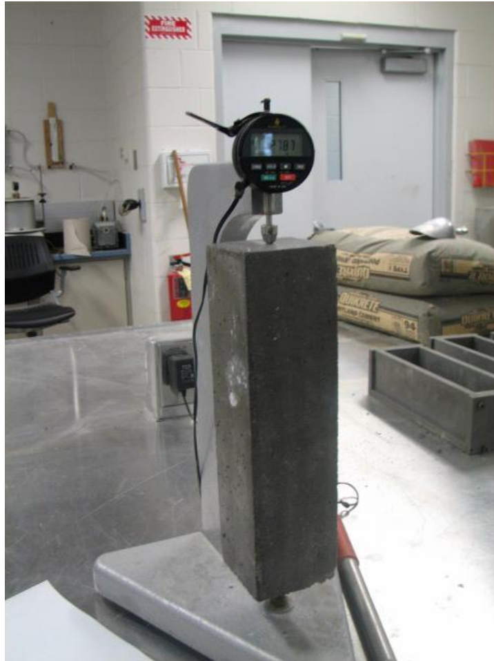
Figure 6.3.2.1 length change, comparator reading
