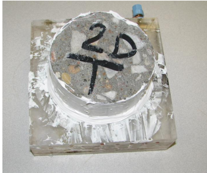
Figure 6.3.3.1 Chloride ion penetration, test Specimen mix 2D
