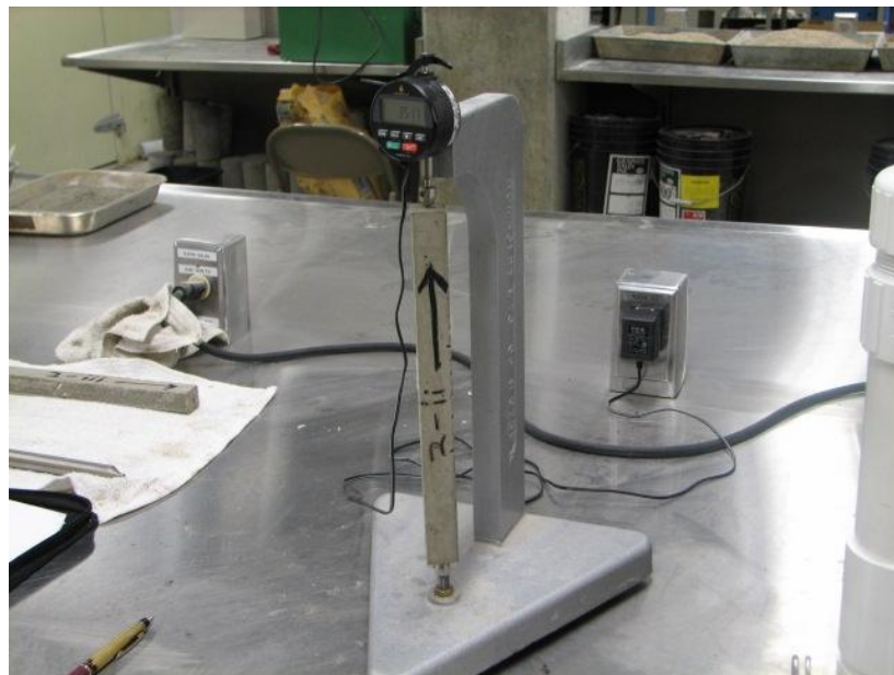
Figure 5.2.5 Taking Comparator Reading of Mortar Bar
