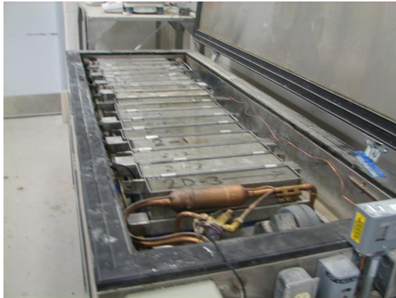
Figure 6.3.1.1 Freeze and Thaw cabinet
