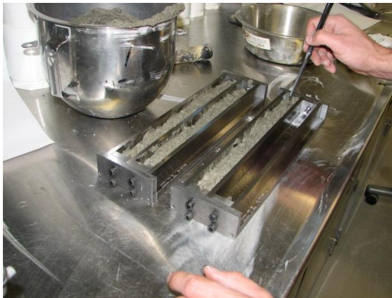
Figure 5.2.2 Casting of Mortar Bars
