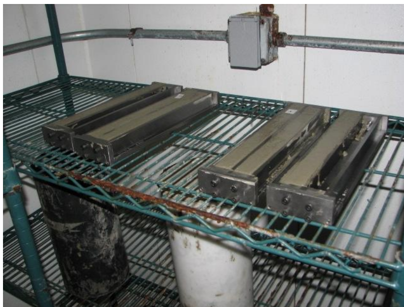
Figure 5.2.3 Initial Curing of Cast Mortar Bars
