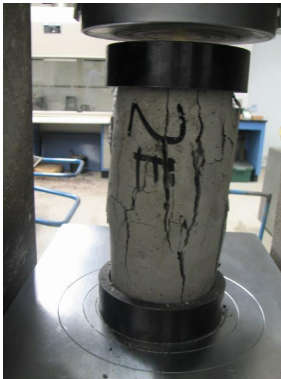
Figure 6.2.1.1 Compressive Strength Testing
