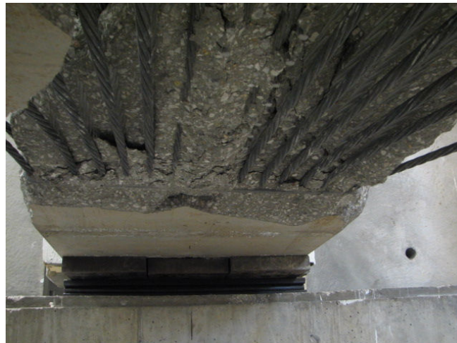
Figure 2.11.4.11: Confined flange non-failed
