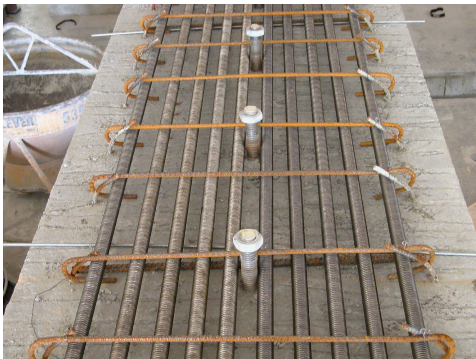
Figure 3.3.3: Common End Plate
