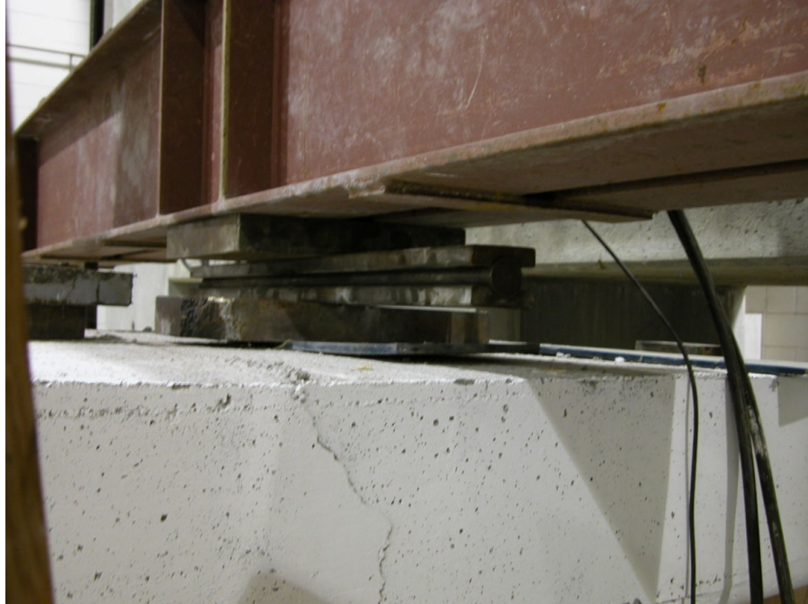
Figure 3.3.25: Add a Roller to Achieve Larger Rotation
