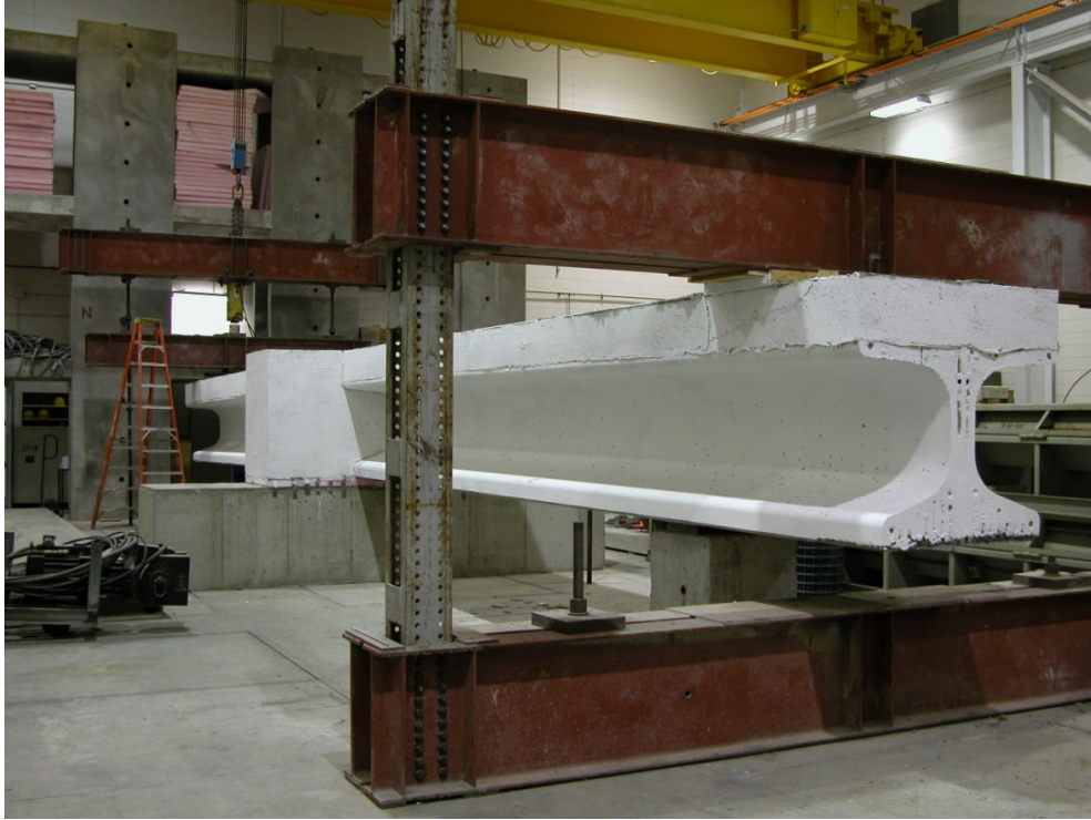
Figure 3.3.19: Passive End of Loading
