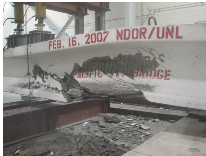
Figure 2.11.4.5: Immediately after shear failure
