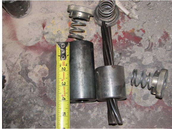
Figure 2.4.2.5: Reusable and one-time use chuck
