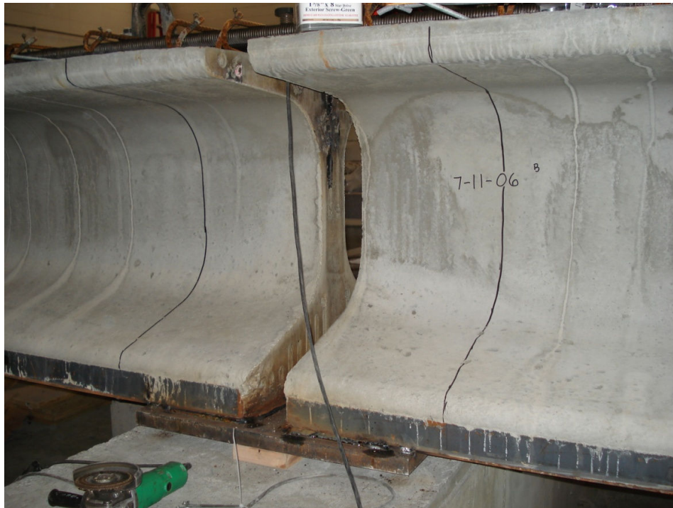
Figure 3.3.5: Welding the Sole Plate and the Shoe Plate Together
