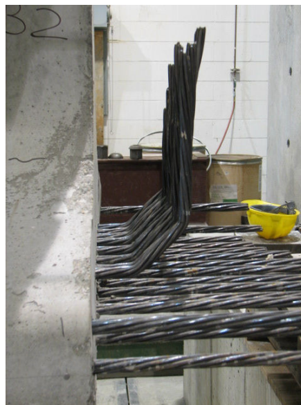
Figure 2.10.2: Second 45 degree strand bend
