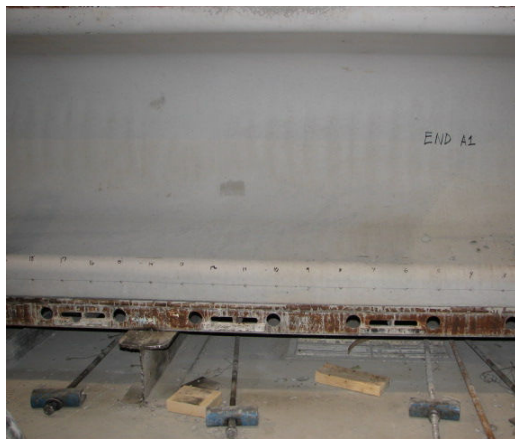
Figure 2.9.1: DEMEC point placement
