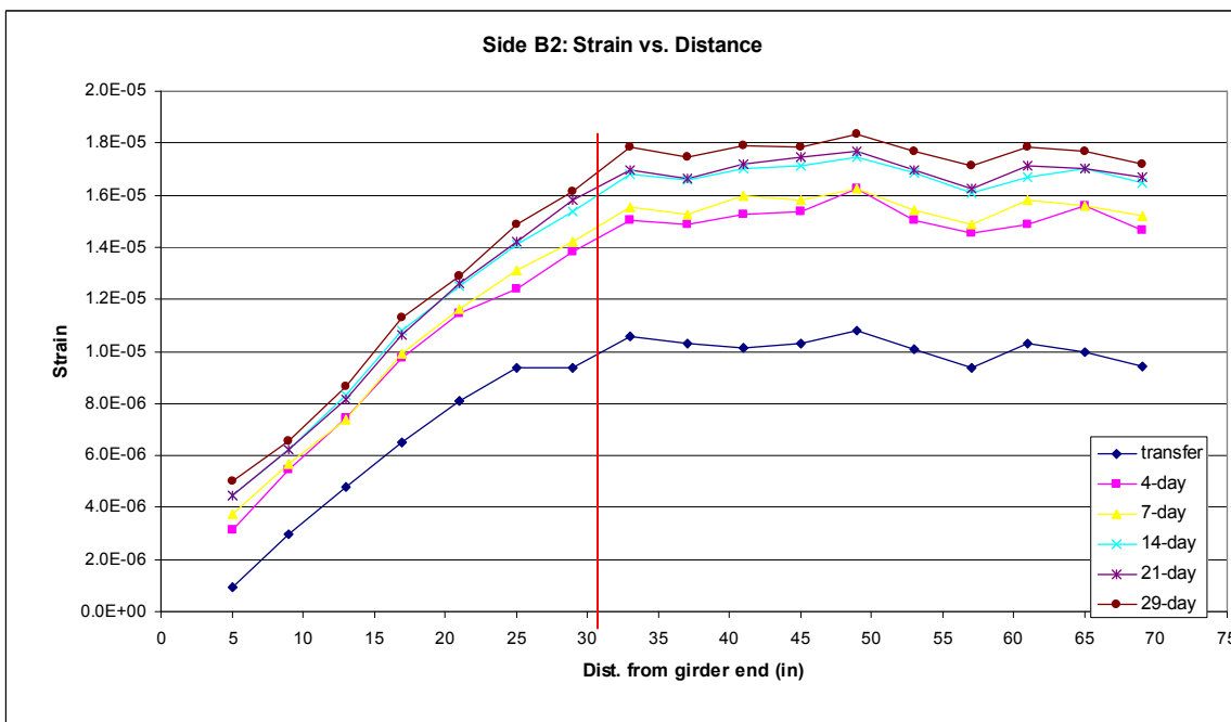
Figure 2.9.7: Side B2 strain versus distance
