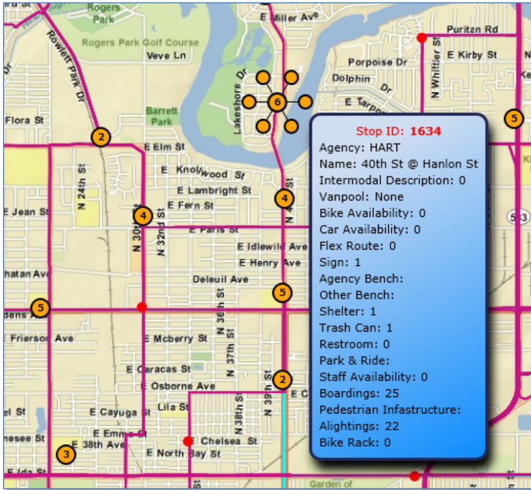
Figure 26 – When user hovers mouse cursor over bus stop, information about stop appears based on data from agency's GTFS feed.
