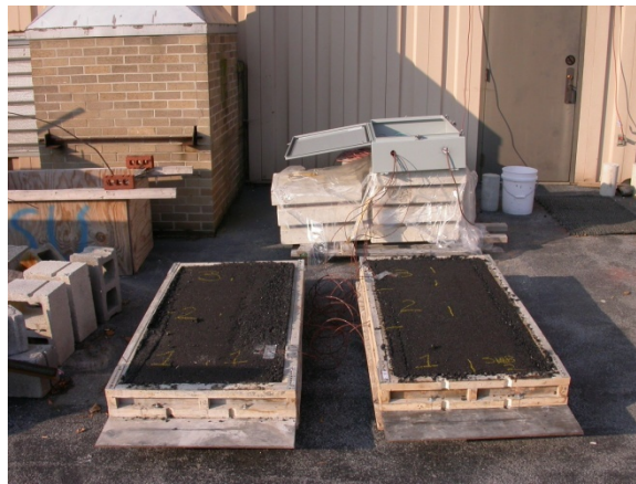
Figure 11. Test slabs exposed to outdoor environment for curing.
