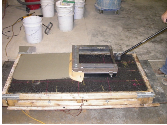
Figure 12. Test slab being coated with Tensar's coating.
