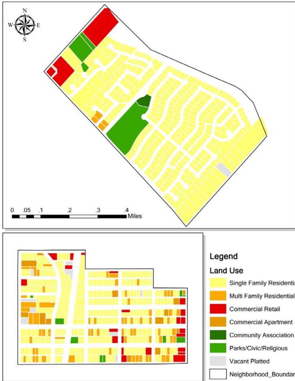
Figure 8: Street Network Density: The Suburban Block Group (Top) Has a Street Density of 2.58, While the Urban Block (Bottom) Has a Street Density of 3.90.
