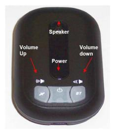
The device used weighs less than 2 ounces. It has a memory of 8 megabytes, and runs on a cell phone battery. The device contains a vibration sensor, which turns the unit off if no vibration is sensed for 15 minutes, but turns the device back on immediately when new vibration is sensed. This serves to save
