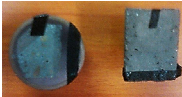
Figure 7. SEM samples for interface examination. Left - polished specimen for profile analysis; Right - unpolished specimen for surface analysis.
