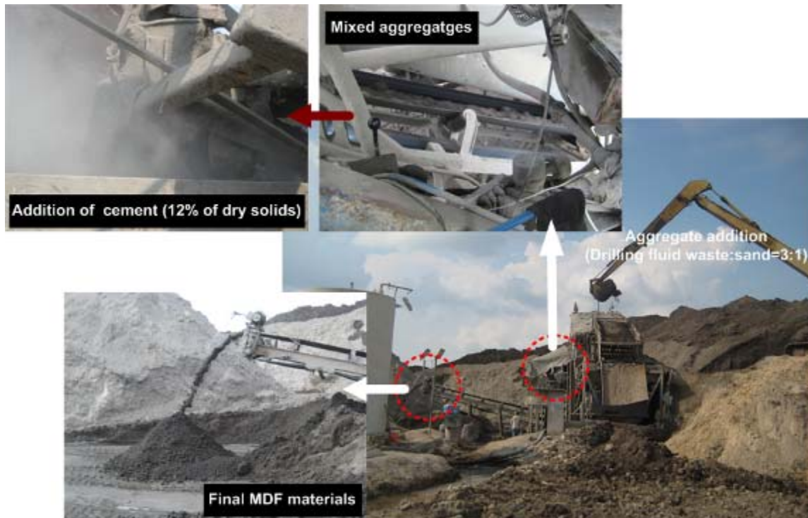
Figure 47. Stabilization and Solidification Processes to Produce MDF Material.
