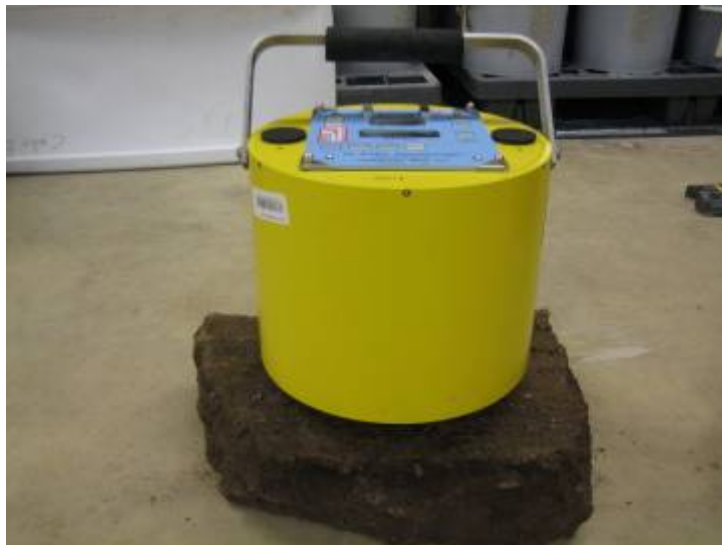
Figure 88. GeoGauge Stiffness Testing.
