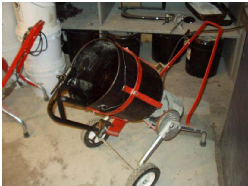
Figure 3-2. Mechanical asphalt mixer
