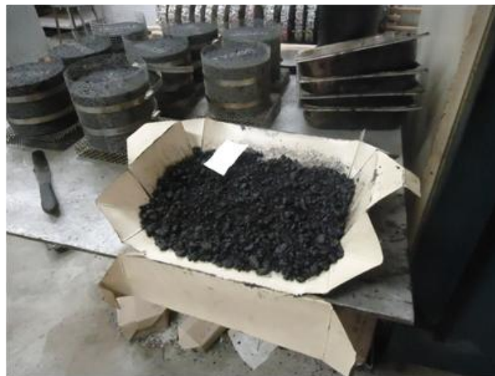
Figure 3-2 Loose mixture for STOA
