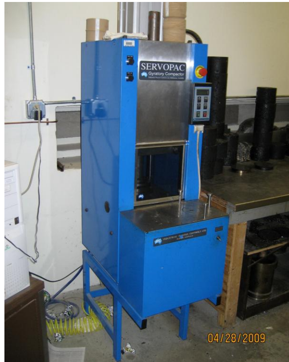
Figure 4-4 Superpave Servopac Gyratory Compactor
