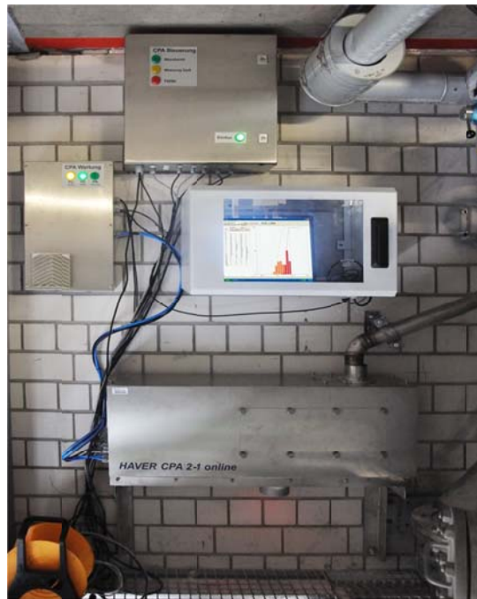
Figure 14 CPA On-Line System to check the Roundness of Plastic Granules
