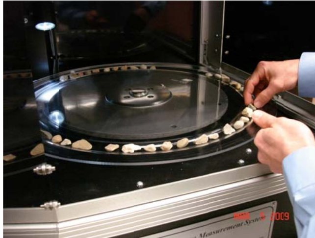
Figure 4 Aggregate Imaging System Modified by Pine Instruments
