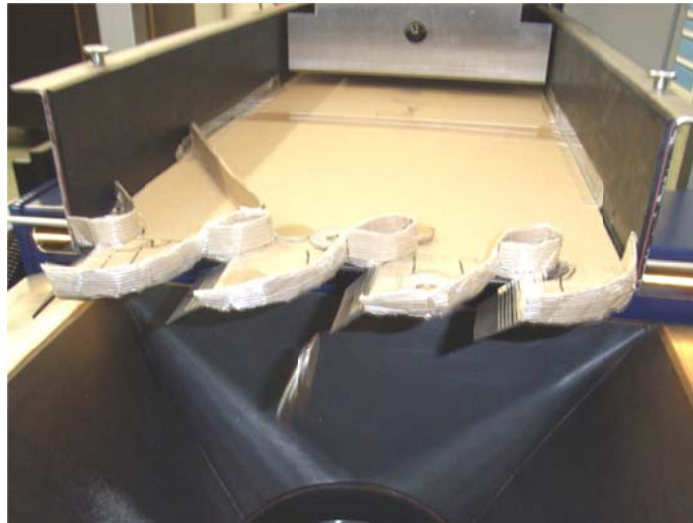
Figure 33 Feeder redesign with Rounded Walls
