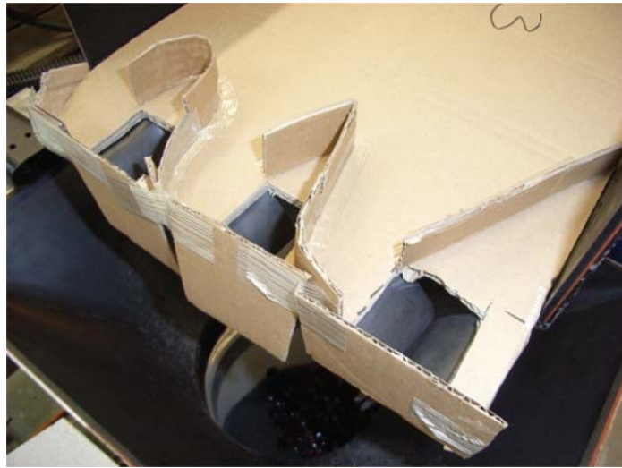
Figure 35 Feeder with Combination of Round and Square Walls
