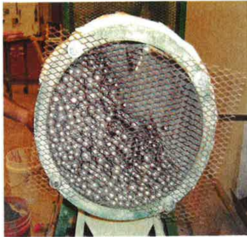
Figure 3.3 Balls motion in the grinding system
