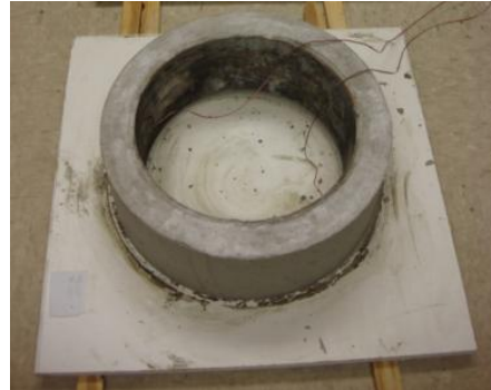
Concrete ring with paraffin wax
