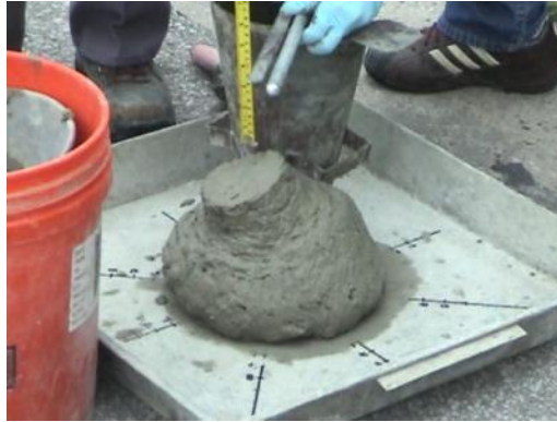
Figure 6–11. Slump of S4TH-M1 after addition of HRWR (40 min after start of mixing)
