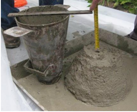
Figure 6-27. Slump of NR-M2-A
