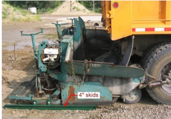
Figure 6–2. Asphalt paver used for slip-form paving
