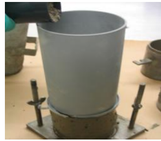
(d) Loading: a big cylinder is placed on top of fresh concrete sample; sand is gradually loaded into cylinder until sample fails
