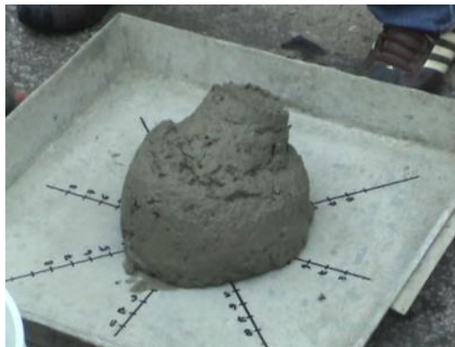
Figure 6–10. Initial slump of S4TH-M1 (30 min after start of mixing)
