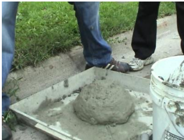
Figure 6–14. Slump of S4TH-M2
