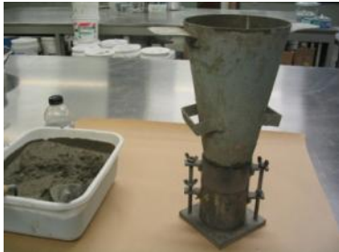
(a) Test setup: slump cone placed on top of a plastic mold without the bottom
