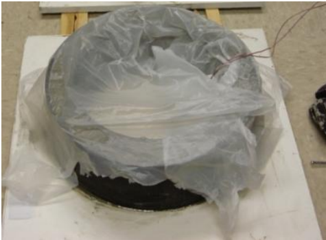
Newly cast concrete ring
