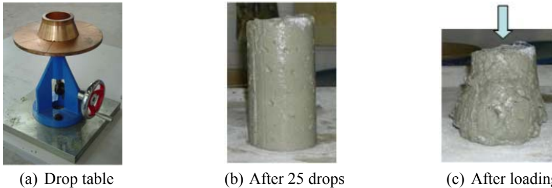
Figure A-4. Device and samples used for modified green strength measurement, Method B
