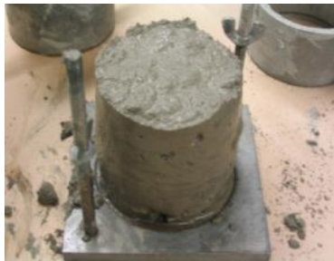
(c) Demolding: after plastic mold is removed; some concrete holds its shape
