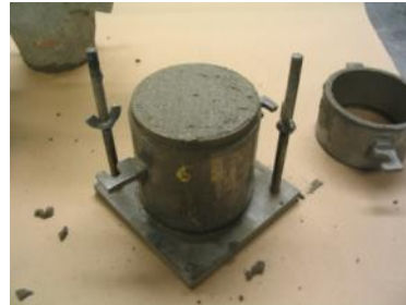
(b) Casting: mold is filled with fresh concrete without rodding or vibration
