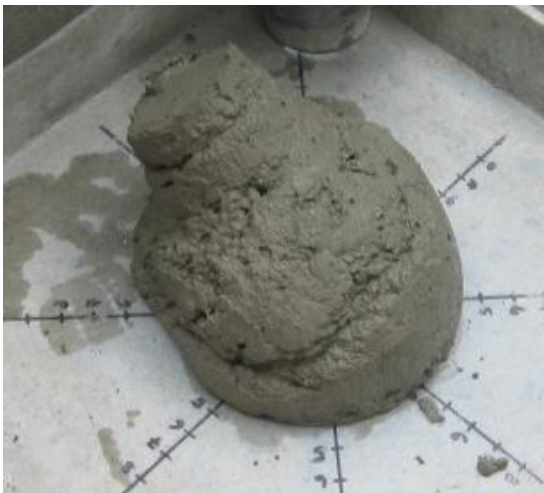
Figure 6-25. Initial slump of NR-M1-A
