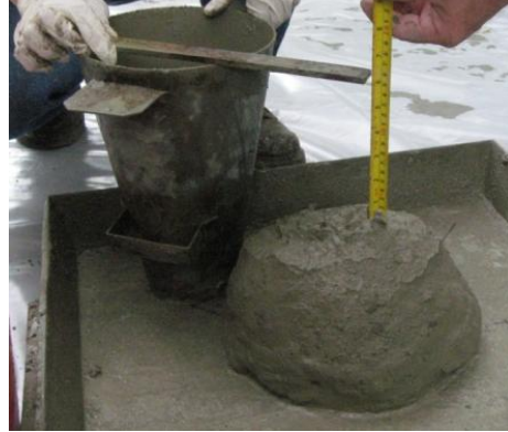
Figure 6-28. Slump of NR-M3-A
