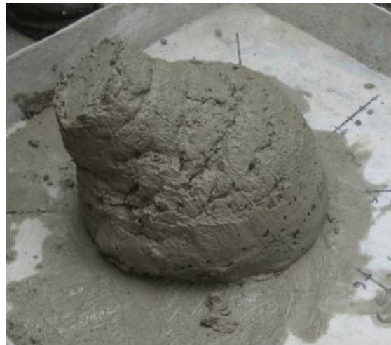
Figure 6-26. Slump of NR-M1-A after addition of HRWR and water
