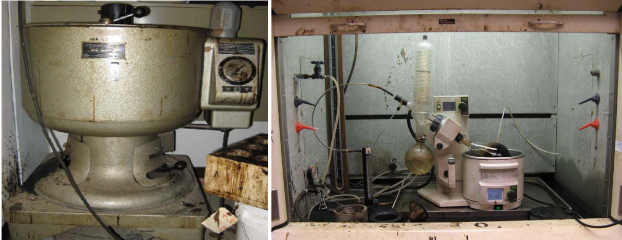
Figure 8. Centrifuge-Rotavapor Recovery Method.
