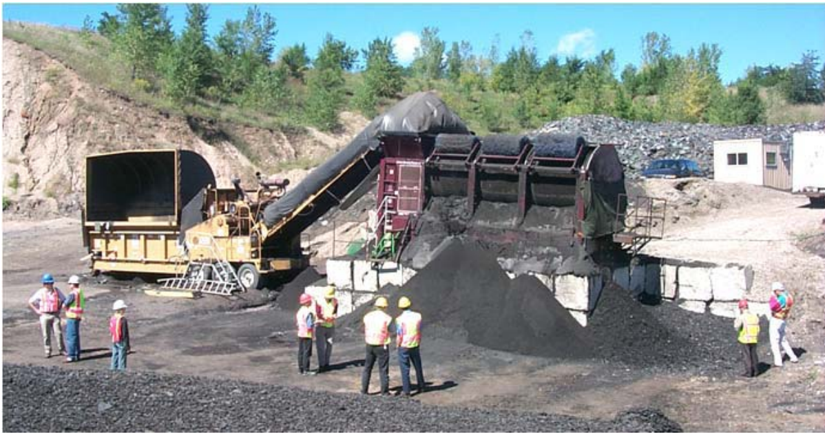
Figure A-3. Shingle Grinder Followed by Trommel Screen (after Krivit, 2007).
