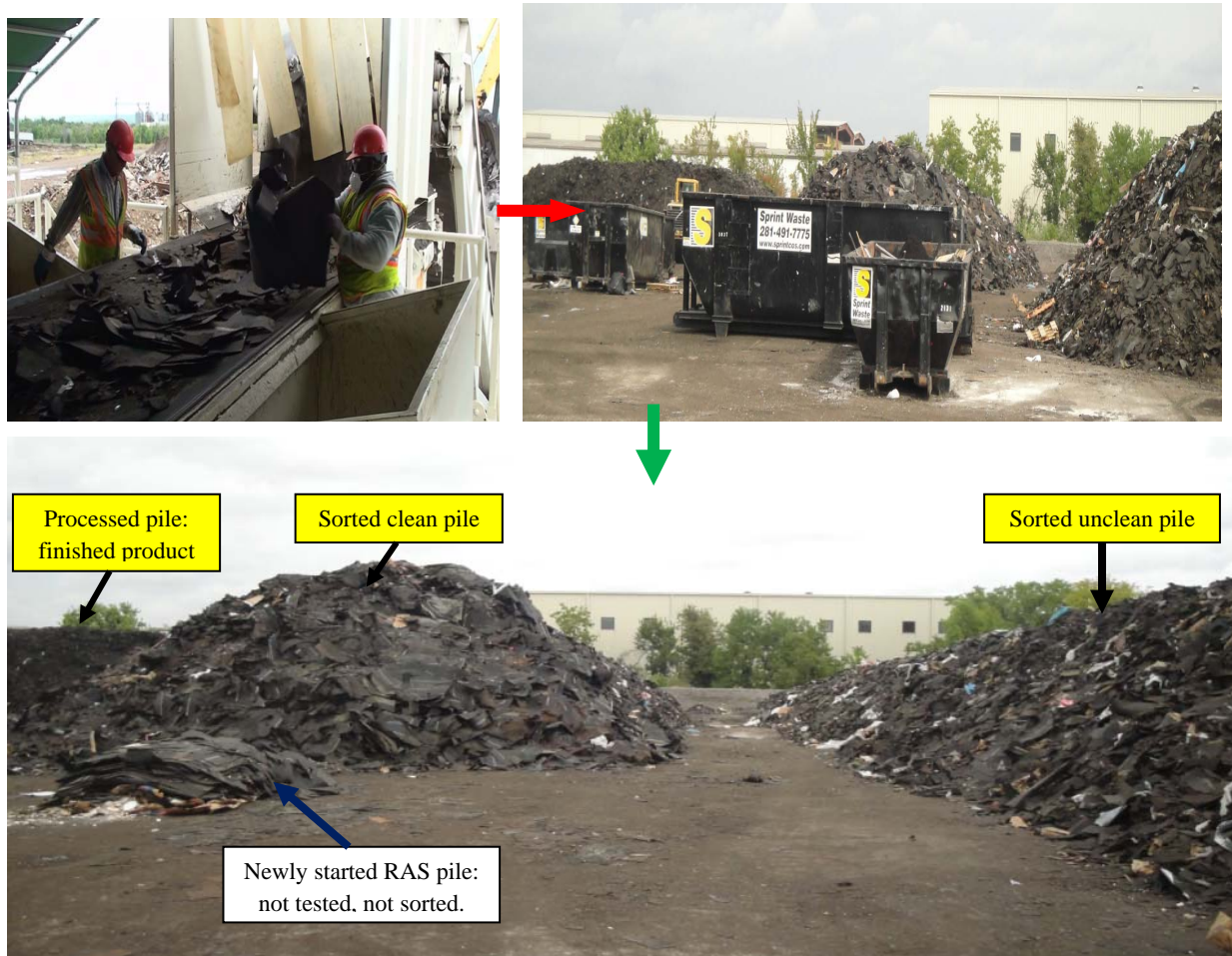
Figure 4. Sorting RAS Manually (Picture (1) one after Krivit, 2007).
