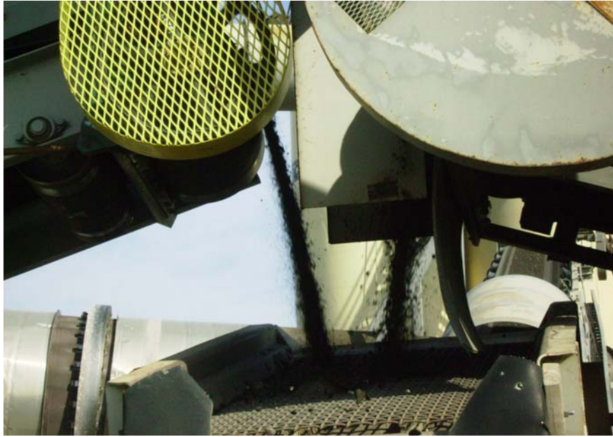
Figure 10. Vibratory Scalping Screen (after Morton, 2011).
