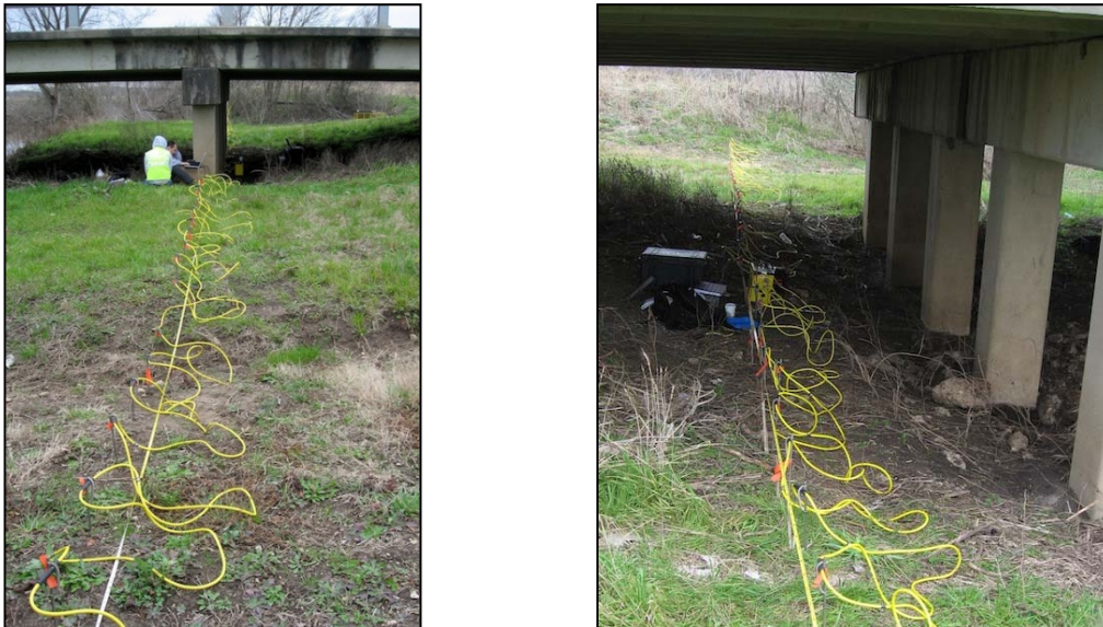
Figure 11-8. Bridge 15 ERI Fieldwork.
