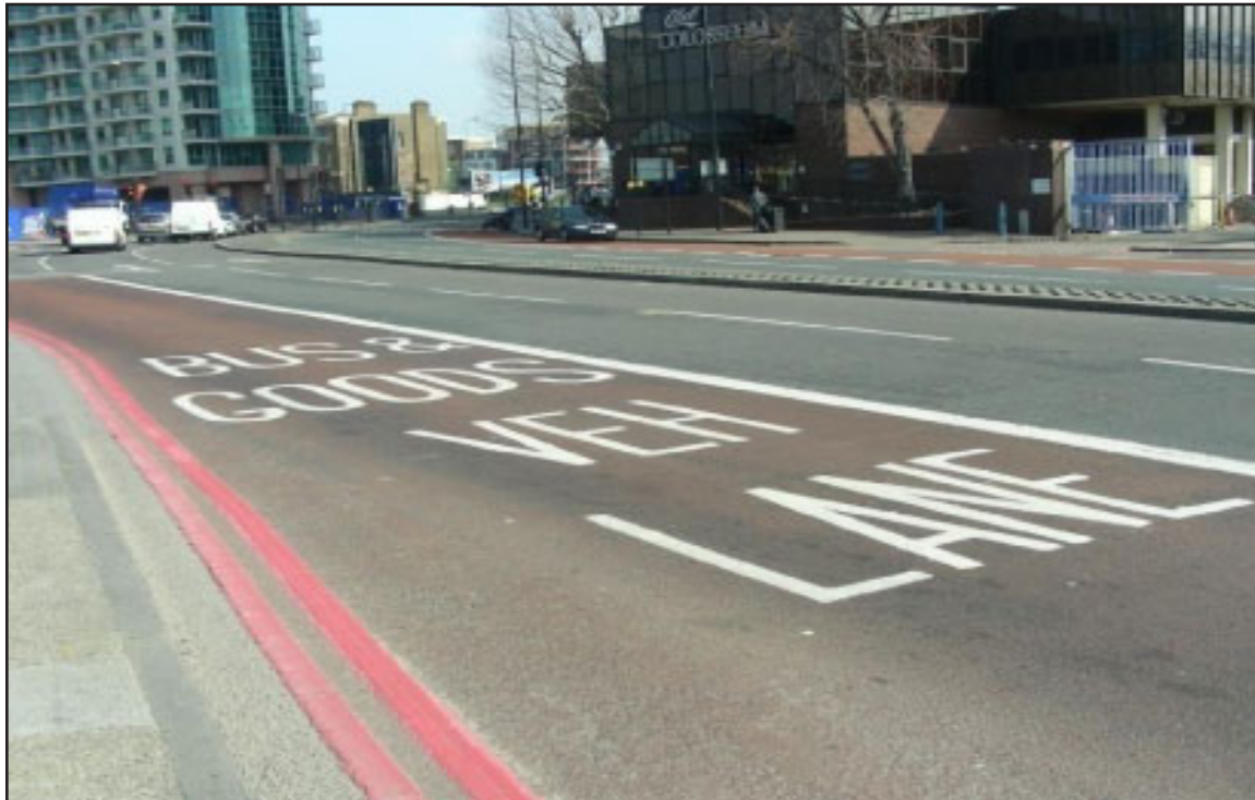
Figure 2. Pavement Text Indicating that Goods Vehicles are Allowed in the Bus Lane (London)
