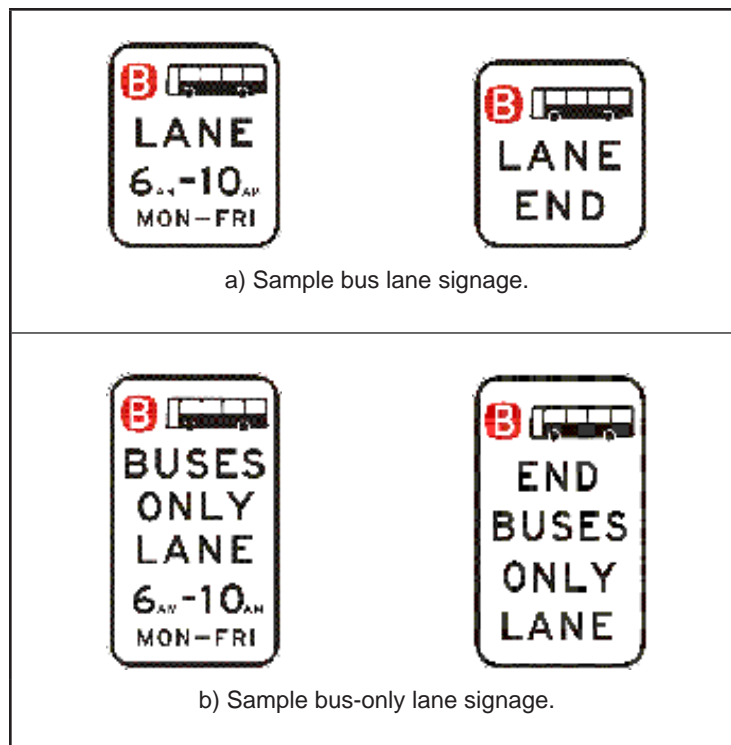
Figure 35. Example Bus Lane and Bus-only Lane Signage (Sydney)
