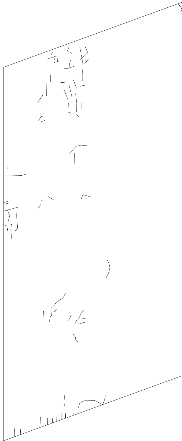
Figure 13 Concrete Slab Bridge Number ASD-89-0294 Crack Map
